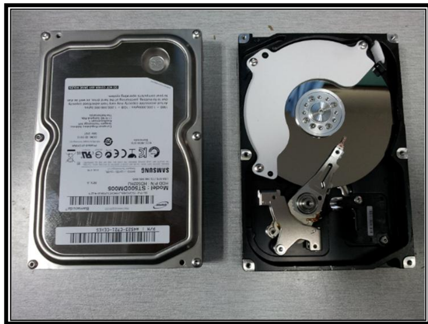
Figure 19: Re-Assembling the Hard Disk Drive (Before and After)
