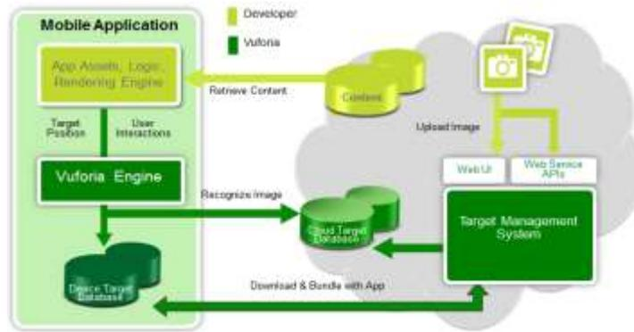
In this program the image targets are downloaded to be used in the device target database (follow the diagram content marked in green), the cloud target database option is excluded and not used in this application, to provide a non-internet dependent working application.
