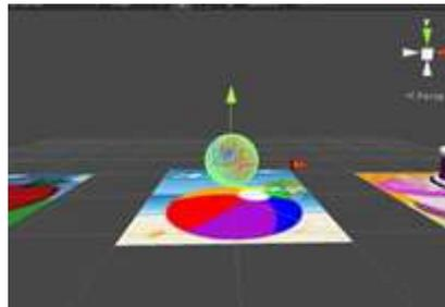
Figure 61 : mesh collider attached to the ball model
