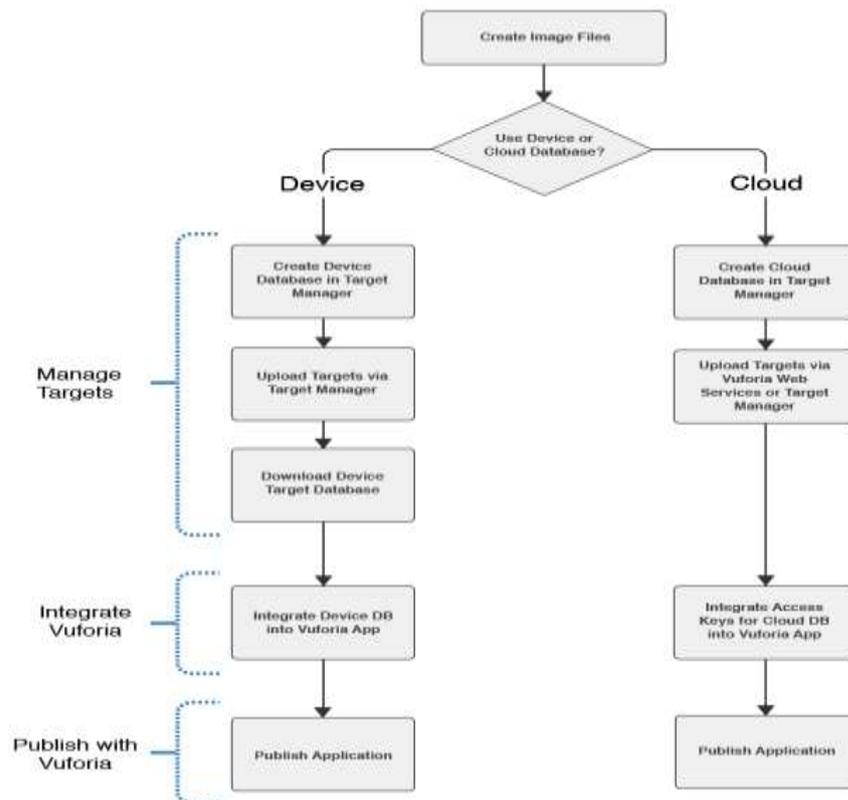
Figure 47 : Vuforia Target markers process flow chart
