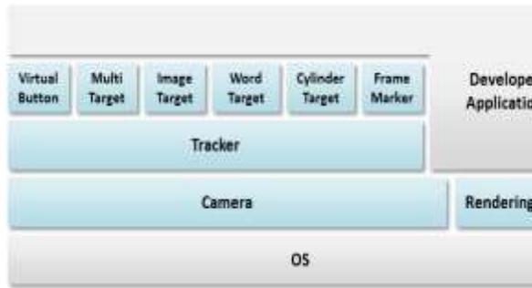
Figure 41:High-level system overview of Vuforia SDK
