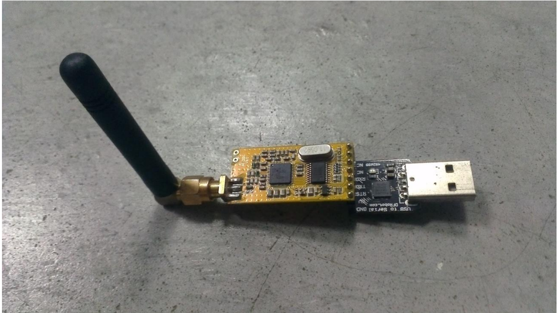
Figure 23: Wireless USB receiver for connection between accident detection device in the vehicle and the computer
