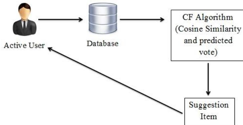
FIGURE 5: System Architecture
