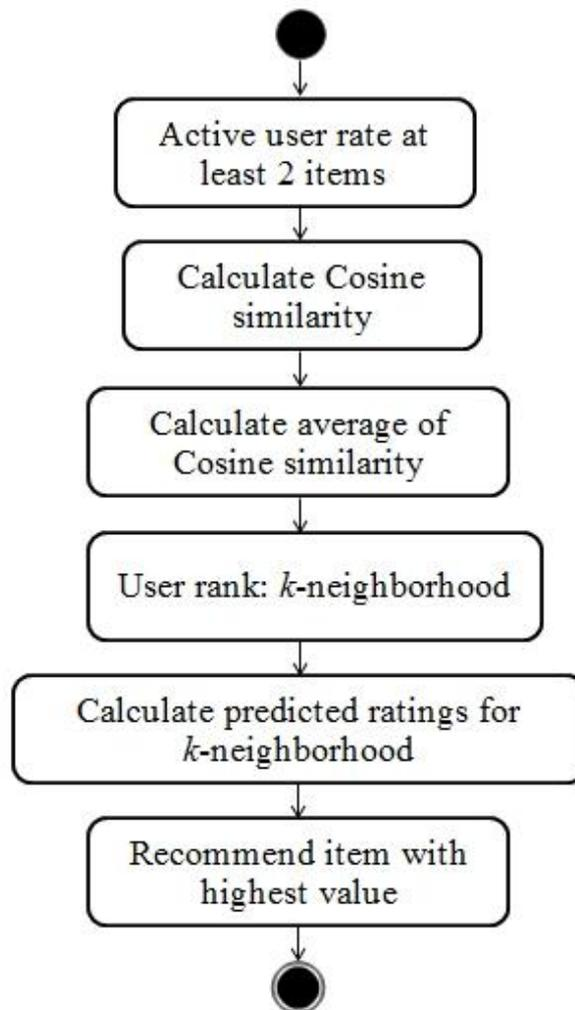
FIGURE 6: System Flow Diagram
