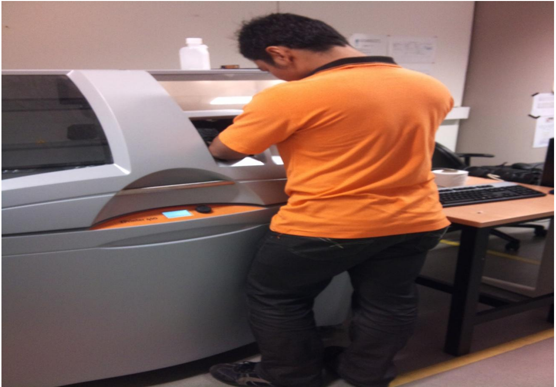
Figure A-3: Using rapid prototyping machine to print designed part for casting the mold
