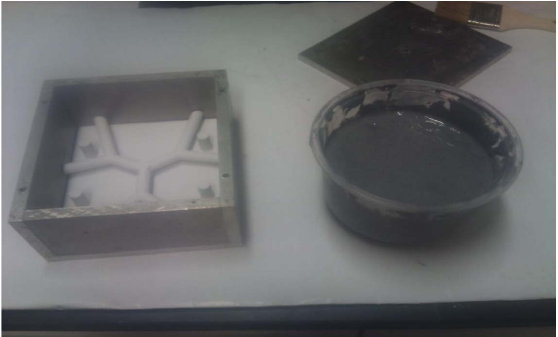
Figure A-7: Epoxy mixture (right) and steel container (left); before epoxy is poured inside the container to cast the mold
