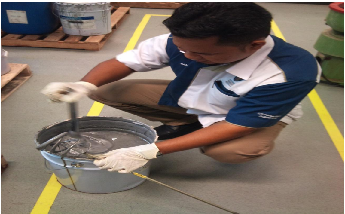
Figure A-6: Stirring the epoxy with metal stick to soften the epoxy
