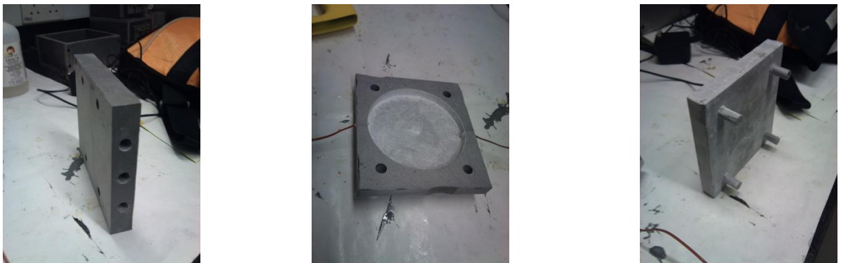
Figure 3.22: Prototype for conventional cooling channel, container, and closer
