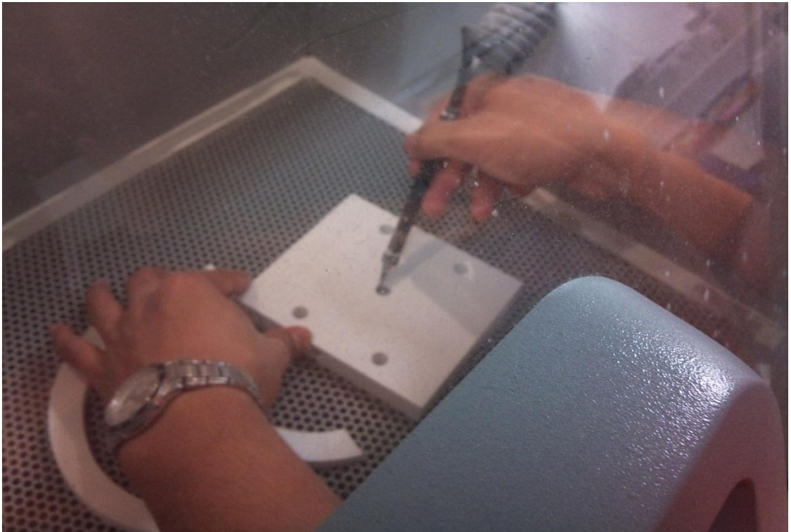
Figure A-4: Using blower to remove the excess powder from the printed part
