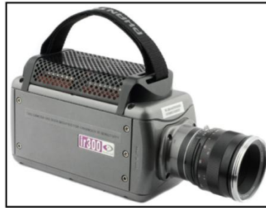
Figure 3.3.5 High speed camera Phantom ir300 model used for the experiment.
