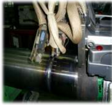
Figure 7: during welding of riser
