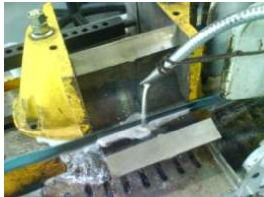
Figure 16: Cutting the pipe into 5 pieces using a linear hack band saw
