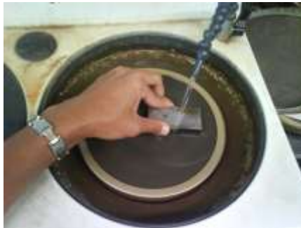
Figure 22: Grinding machine to obtain a smooth and mirror finished surface
