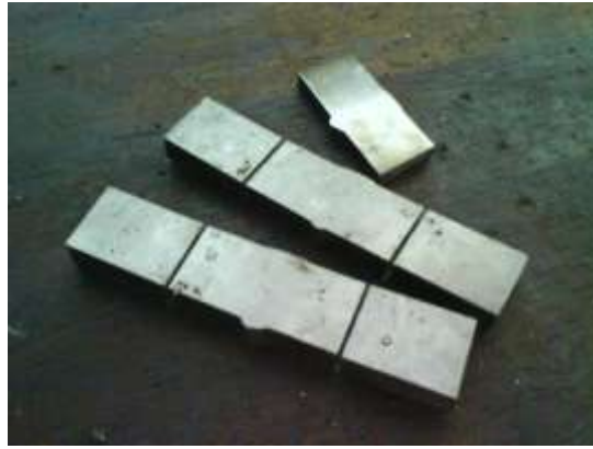
Figure 21: Specimens for hardness test after cutting with linear hack saw machine (top specimen)
