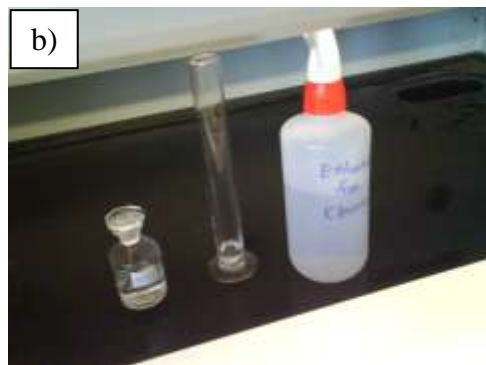
Figure 23: a) Macro-etching lab and b) etchant (diluted nitric acid)
