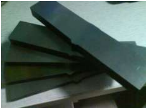
Figure 21: Specimens for hardness test after cutting with linear hack saw machine (top specimen)
