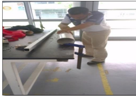
Figure 3.2: One of the technicians does the PVC pipe cutting process using cutter. The PVC pipe is cut into half.
