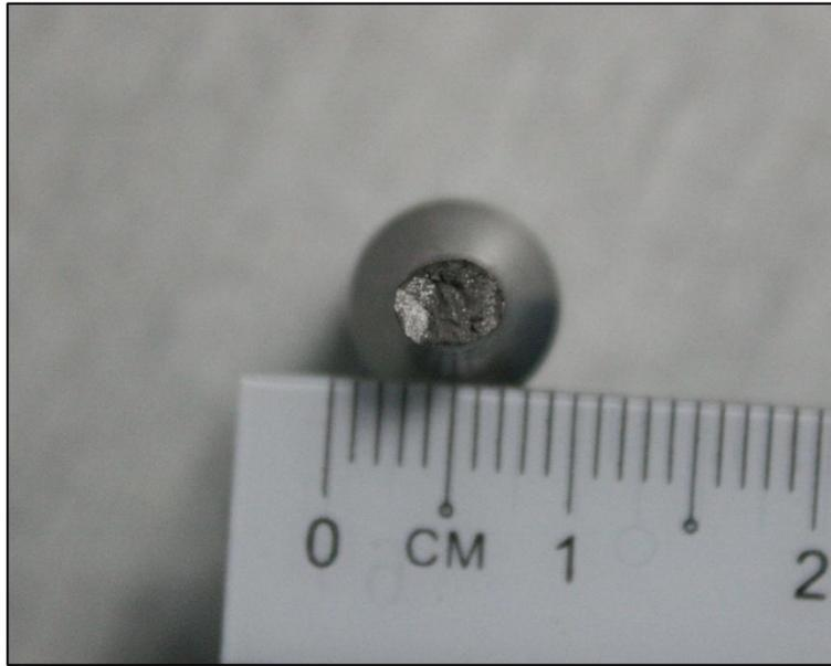
Figure 5.14 Fracture surface of non nitrided specimen under 40 N cyclic loading
