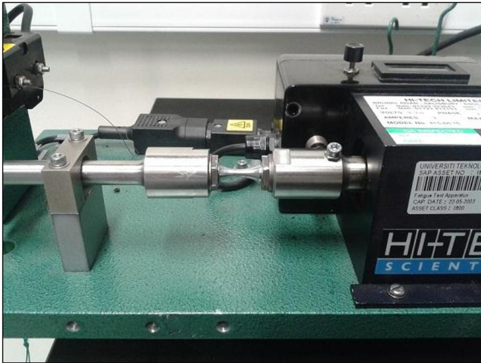
Figure 5.3 Specimen being loaded into the rotating fatigue machine
