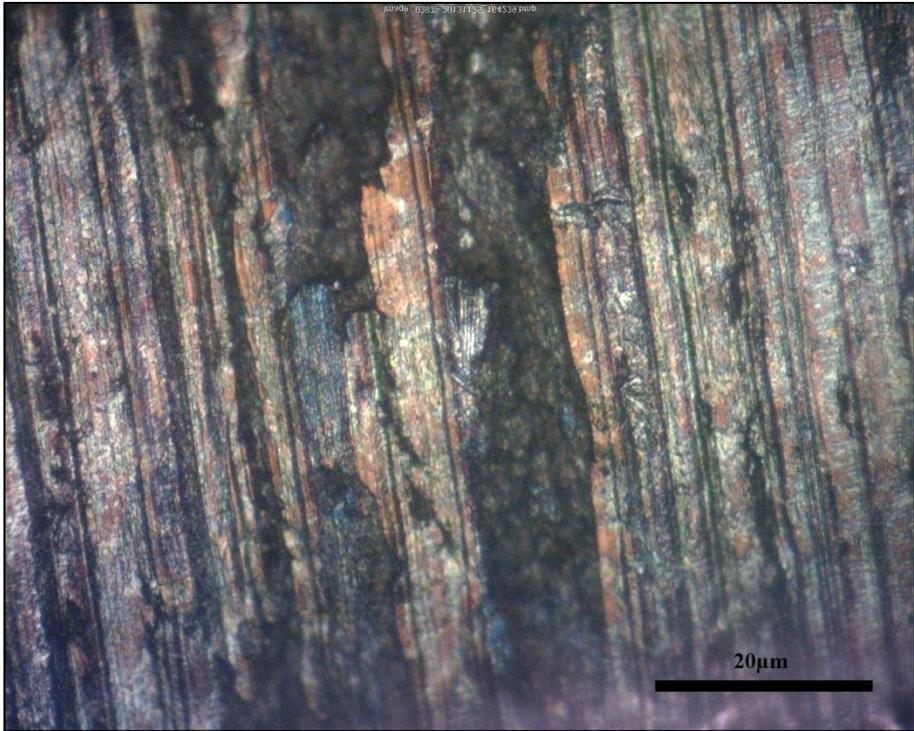
Figure 5.10 Low temperature nitrated specimen after cyclic loading being applied for approximately 50000 cycles under 40 N loads
