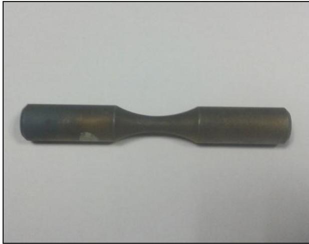
Figure 5.2 High temperature nitrided specimen
