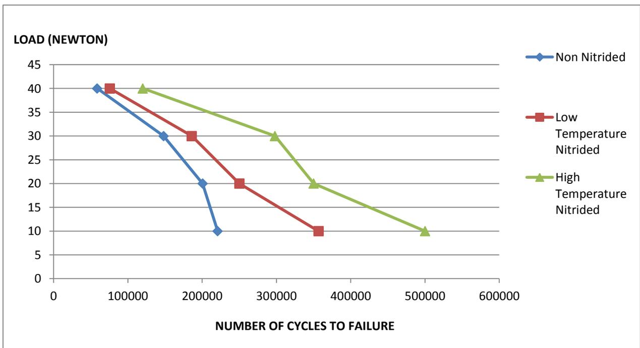
Based on the results for all the three types of specimens, the higher the cyclic loading being applied the lower the number of cycles to failure.
