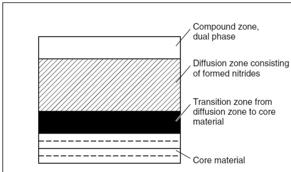
FIGURE 2.2 Typical nitrided case structures [18]
