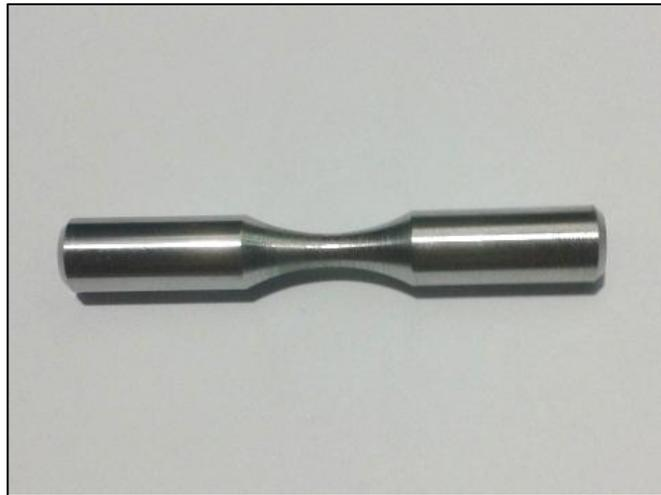
FIGURE 4.1 Stainless steel 439 fatigue specimen
