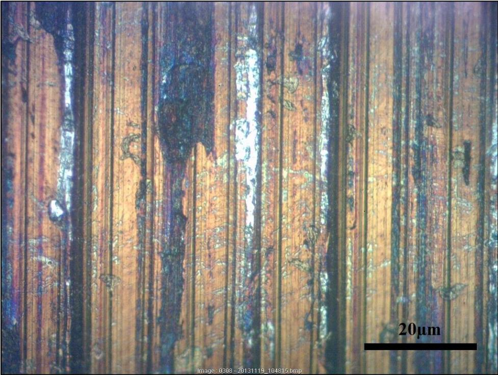
Figure 5.8 Low temperature nitrided specimen before cyclic loading being applied
