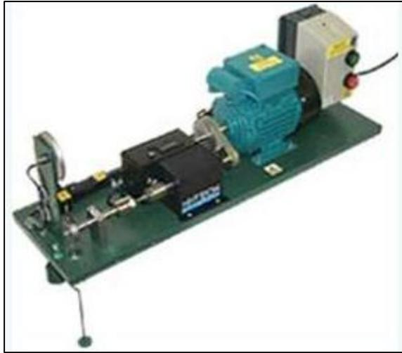
FIGURE 3.3 Rotating fatigue machine
