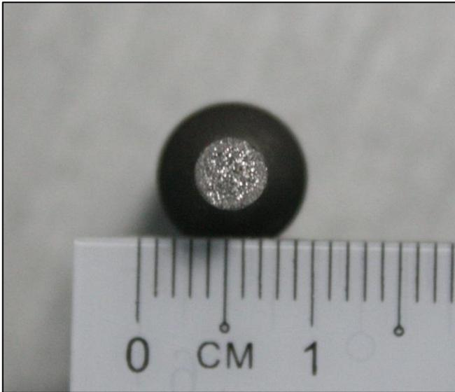
Figure 5.18 Fracture surface of high temperature nitrided specimen under 40 N cyclic loading
