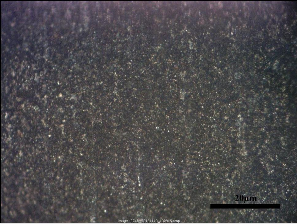
Figure 5.11 High temperature nitrided specimen before cyclic loading being applied
