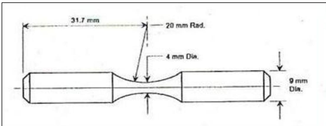
FIGURE 3.2 Fatigue specimen
