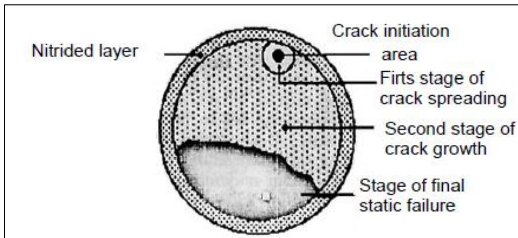
FIGURE 2.3 Scheme of fatigue fracture with near surface initiation of a crack [19]
