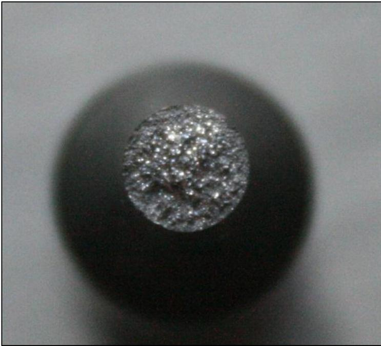
Figure 5.19 Fracture surface of high temperature nitrided specimen under 40 N cyclic loading
