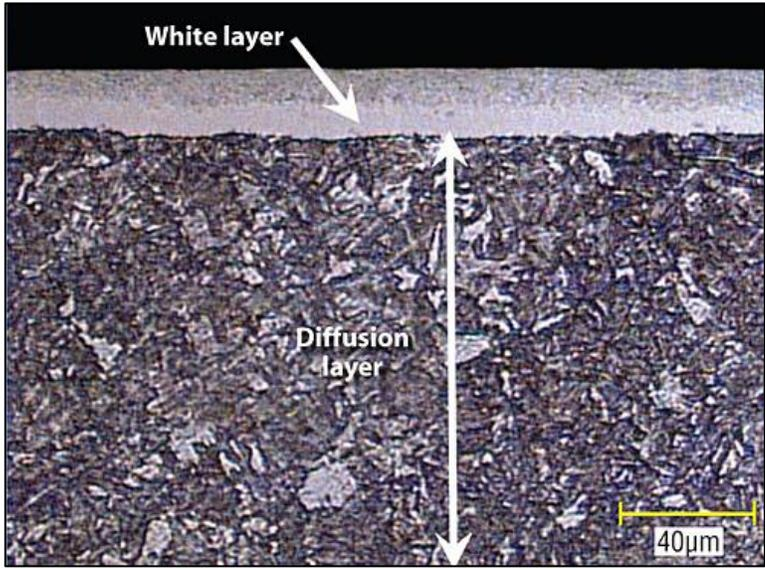
FIGURE 3.4 Typical image of nitrided case structure of a specimen under stereoscopic microscope [14]
