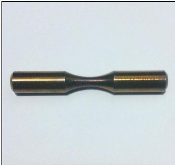
Figure 5.1 Low temperature nitrided specimen
