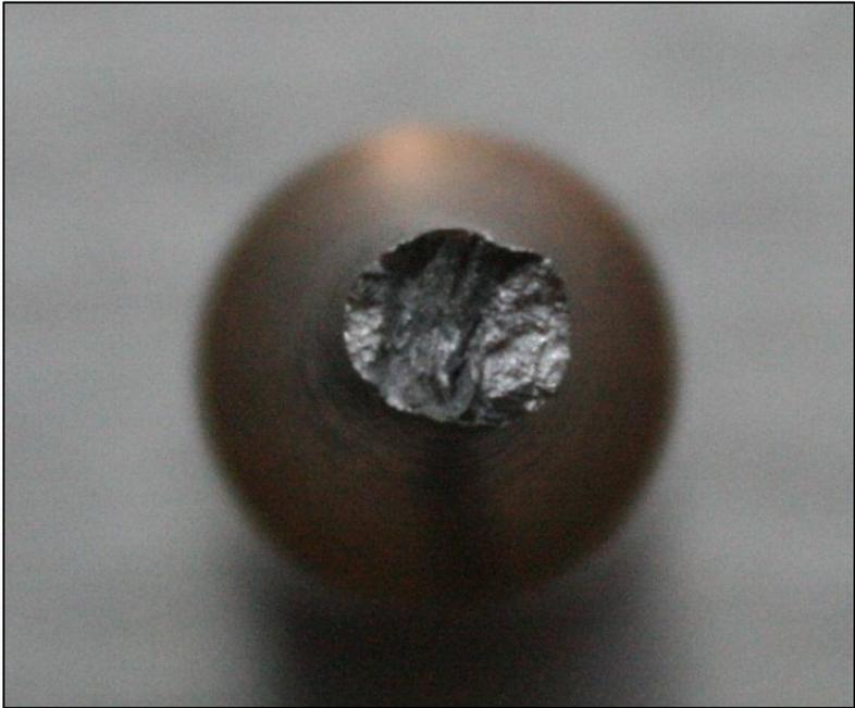
Figure 5.17 Fracture surface of low temperature nitrided specimen under 40 N cyclic loading
