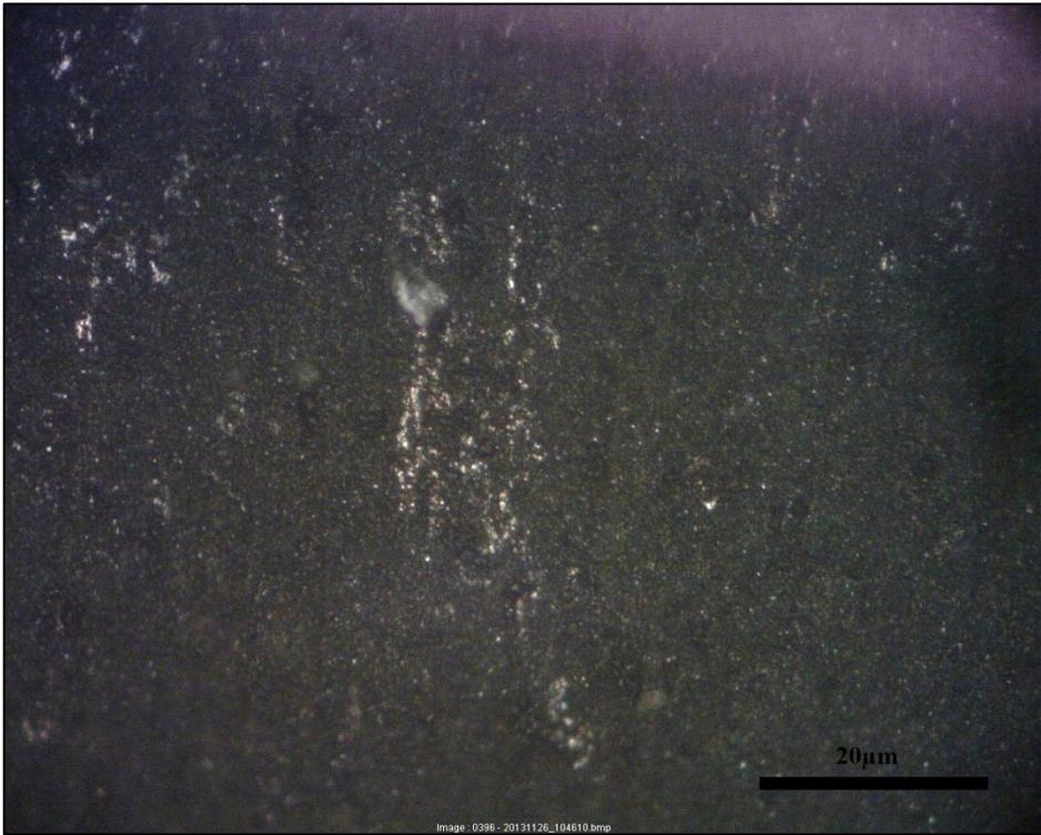
Figure 5.13 High temperature nitrided specimen after cyclic loading being applied for approximately 50000 cycles under 40 N loads
