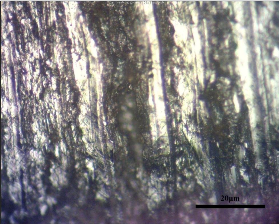
Figure 5.6 Non nitrided specimen surface after cyclic loading being applied for approximately 35000 numbers of cycles
