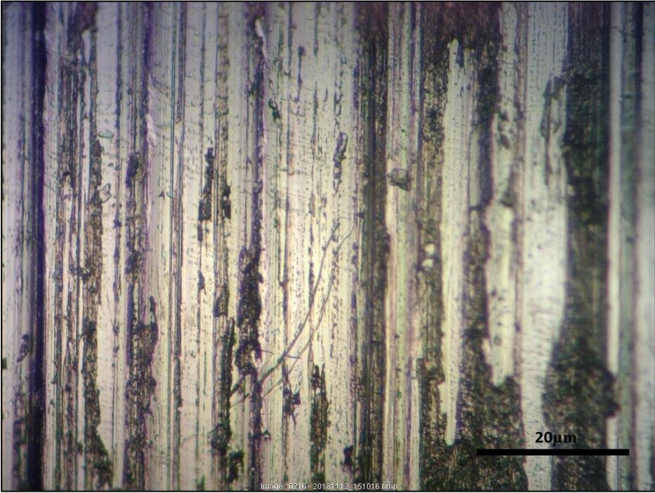
Figure 5.5 Non nitrated specimen surface before cyclic loading being applied
