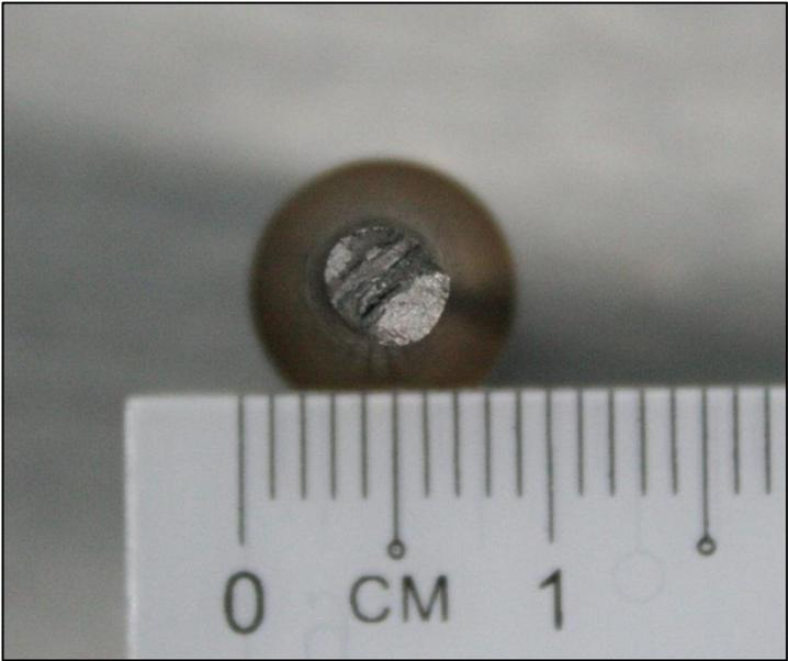
Figure 5.16 Fracture surface of low temperature nitrided specimen under 40 N cyclic loading
