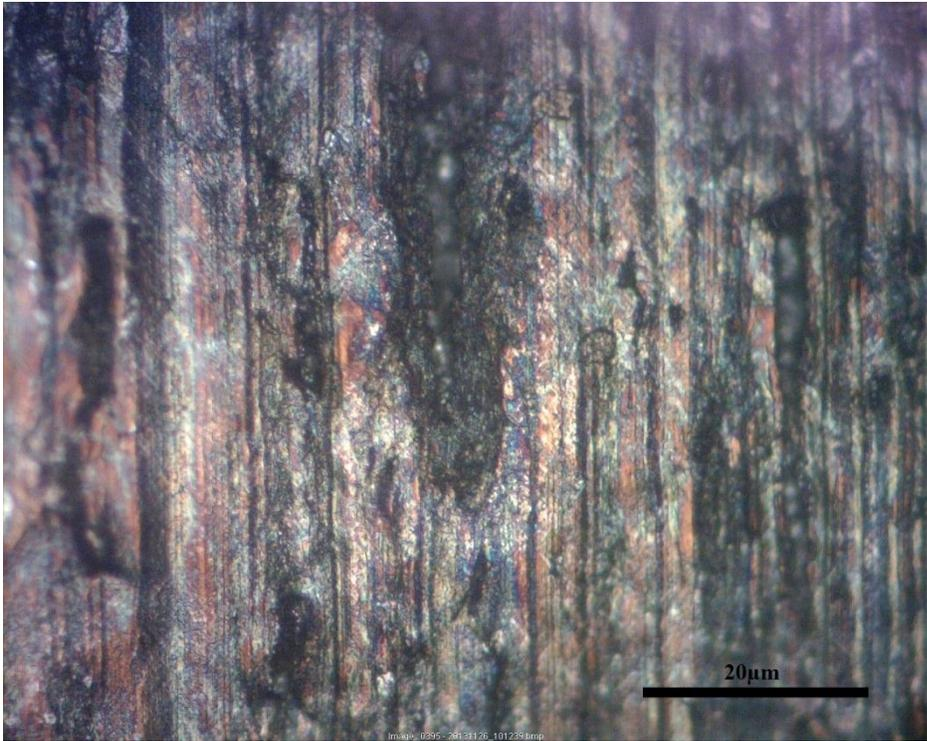
Figure 5.9 Low temperature nitrated specimen after cyclic loading being applied for approximately 35000 cycles under 40 N loads
