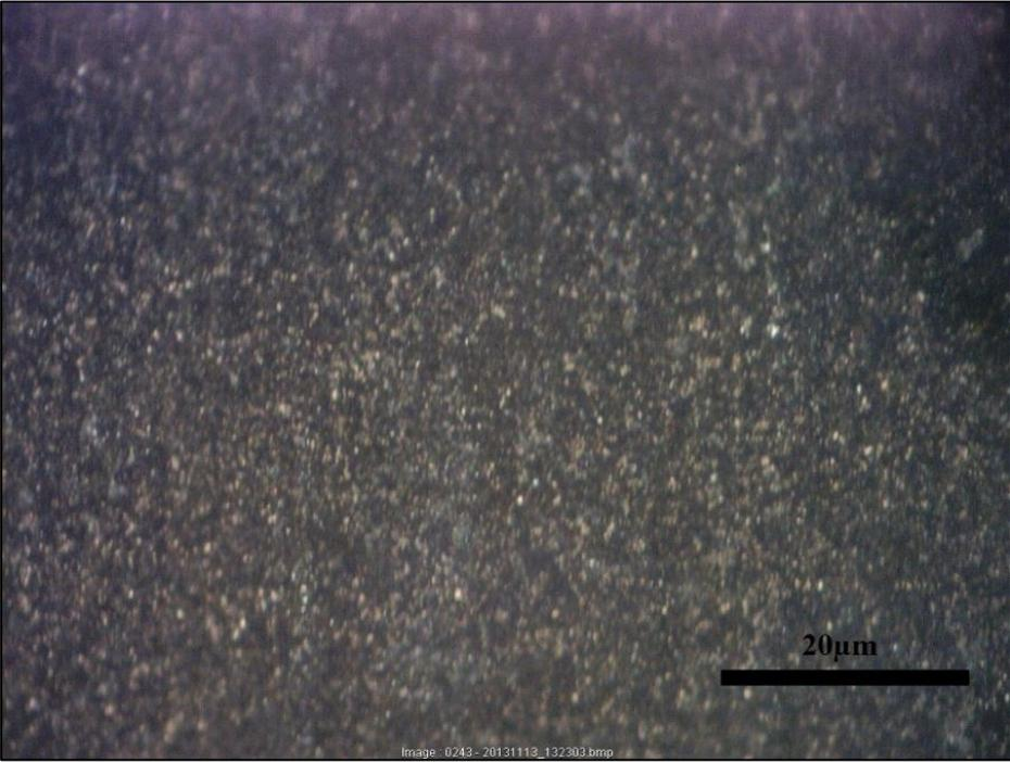
Figure 5.12 High temperature nitrided specimen after cyclic loading being applied for approximately 35000 number of cycles
