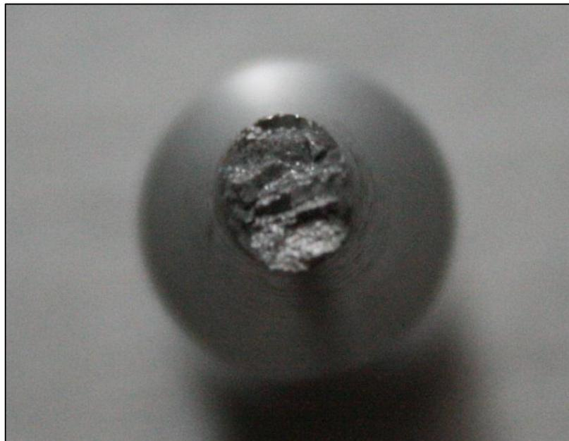
Figure 5.15 Fracture surface of non nitrided specimen under 40 N cyclic loading
