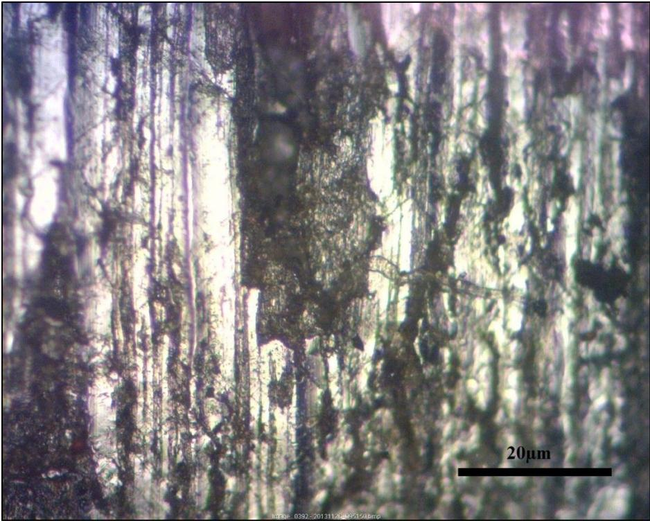
Figure 5.7 Non nitrided specimen surface after cyclic loading being applied for approximately 50000 cycles under 40 N loads
