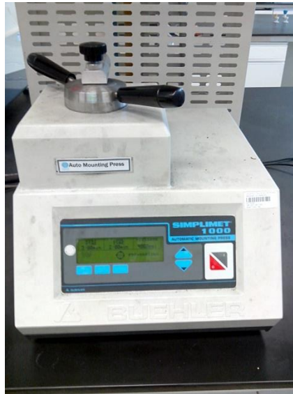
Figure 11: Auto Mounting Press machine used for mounting the samples
