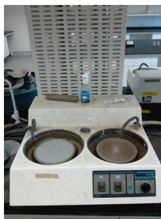
Figure 13: Grinding and Polishing Machine used for surface finishing of the samples
