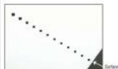
Figure 16: Case depth measurement. The increasing size of the indentations towards the centre of specimen indicate decreasing hardness of the material.
