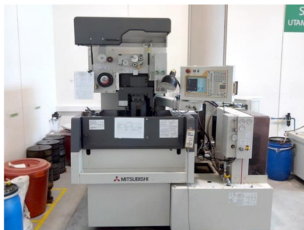
Figure 9: EDM Wire Cut Machine used for cutting the samples
