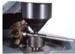
Figure 24: Special anvil for cylindrical surfaces
