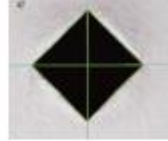
Figure 5. Vickers indents on a smooth surface. 602-Plus DuPro Plus, 50µm. a) Hardened steel, 775 HV 10. b) 0.2% carbon steel, 180 HV 10.
