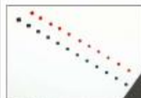
Figure 17: Indents forming a zig-zag pattern.
