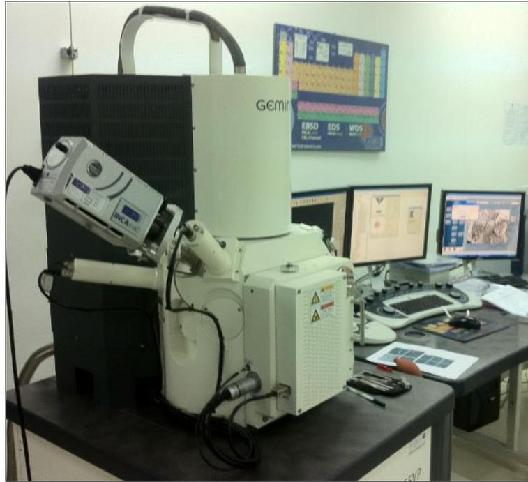
Figure 17: Scanning Electron Microscope (SEM)
