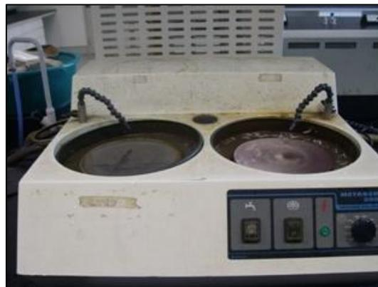
Figure 13: Grinding and Polishing Machine
