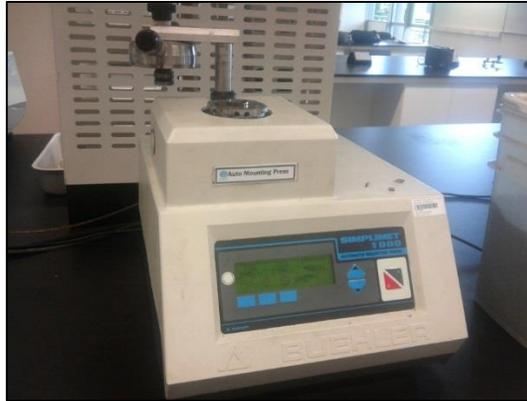
Figure 12: Hot Mounting Press Machine
