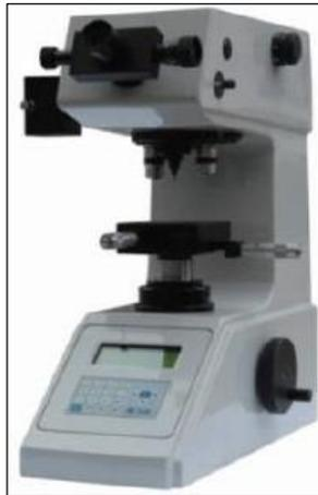
Figure 18: Vickers Microhardness Test
