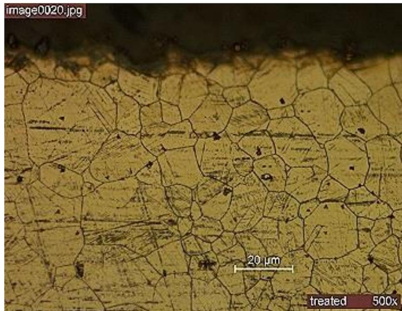
Figure 21: Optical Microscopic of 600°C Nitrided 316L ASS at 500x
