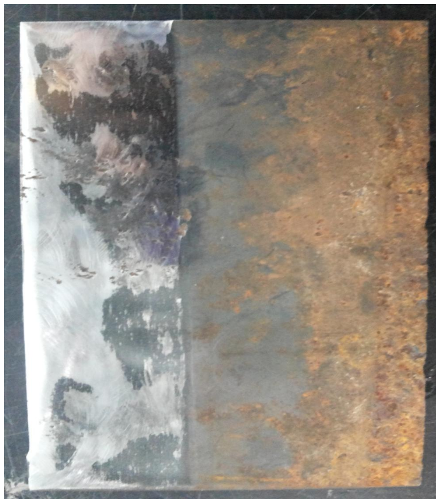
Figure 48. A plate with a section of corroded area
