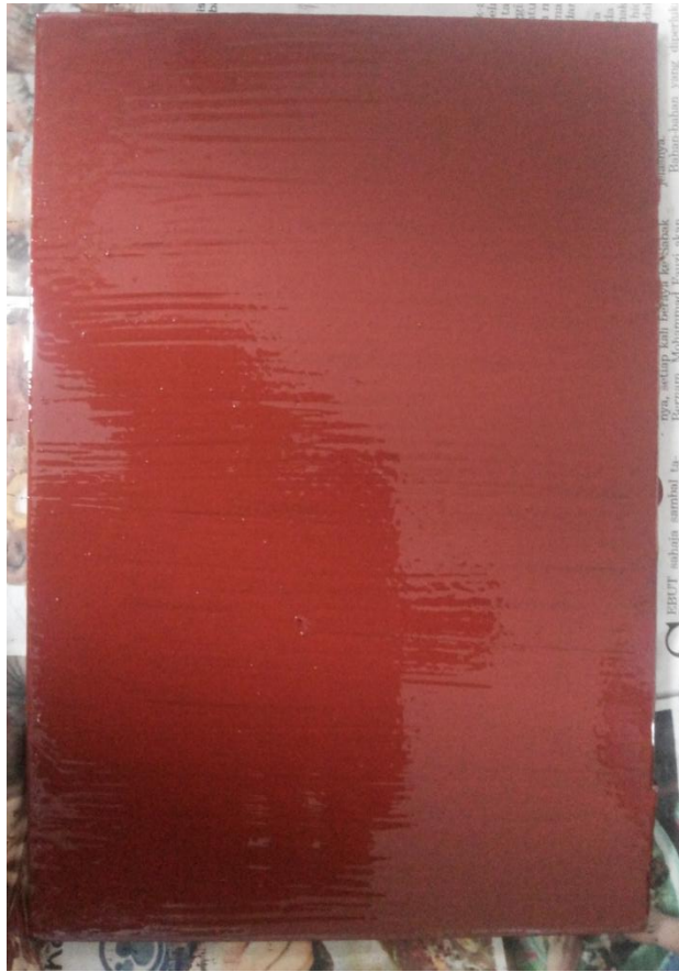
Figure 9. Steel painted with red oxide primer paint
