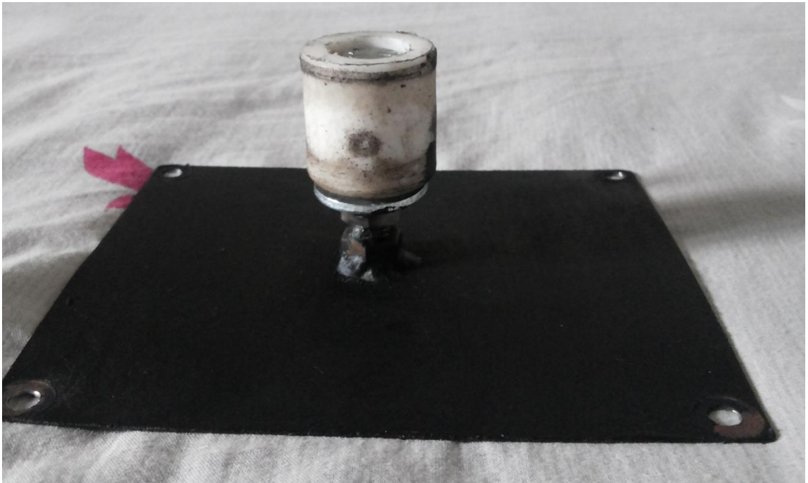
Figure 25. Platform of the camera with roller to enable the platform to move along the railing.
