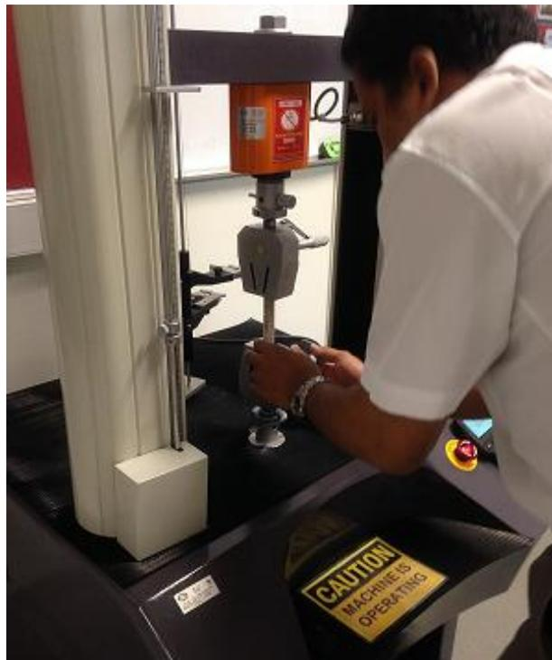
Figure 3.13: The sample is loaded into the tensile grip.
