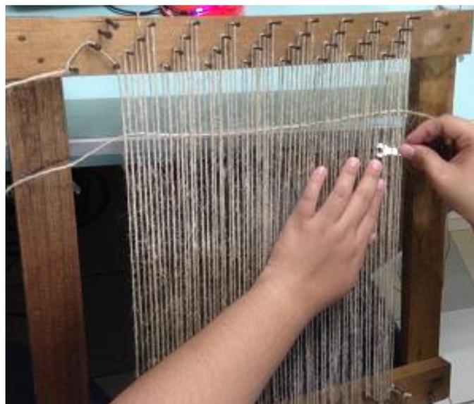
Figure 3.2: Kenaf fibre is weaved using the weaving board.
