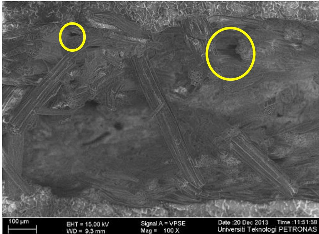
Figure 4.4: FESEM of untreated composite at magnification of 100X.
