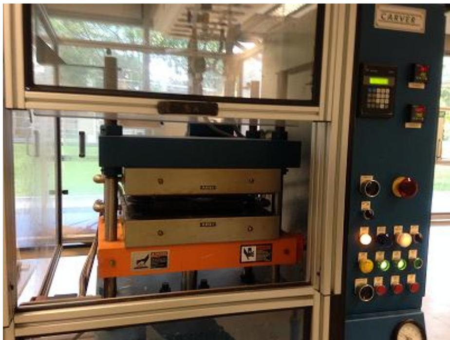
Figure 3.8: The mould is being cooled under compaction.
