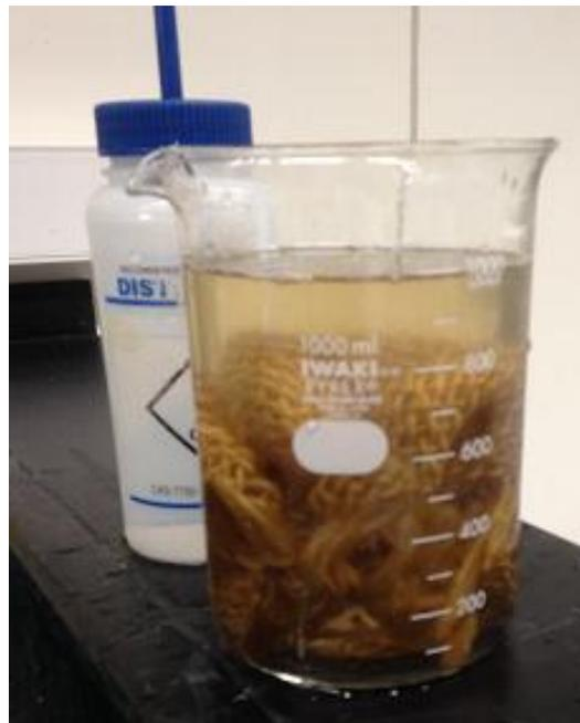
Figure 3.5: Woven kenaf being immersed in 1% concentration acetic acid solution.
