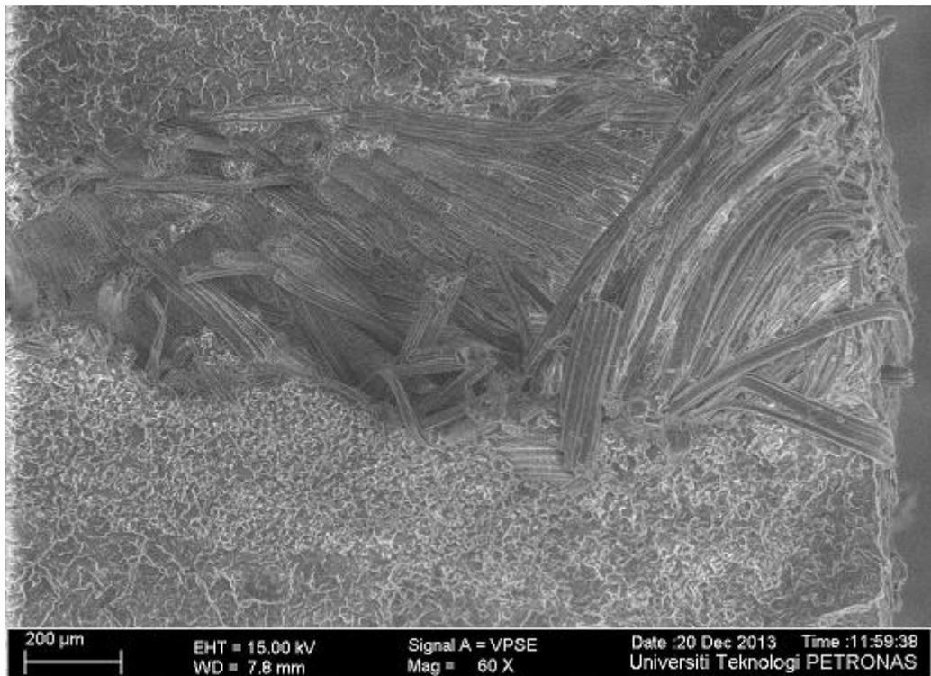
Figure 4.7: FESEM of treated composite at 60 X magnification.
