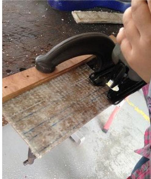
Figure 3.10: The marked composites are cut into rectangular shapes.
