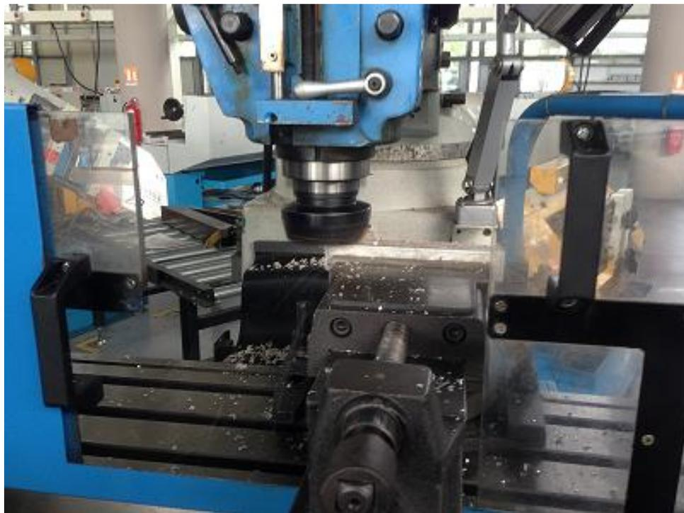
Figure 3.11: The samples are milled in order to obtain required width and length.
