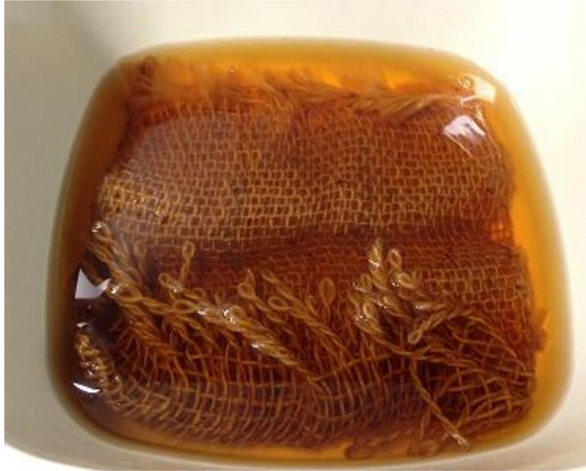
Figure 3.4: Woven kenaf after being immersed in 5% NaOH solution for 24 hours.
