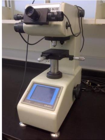
Figure 3.5: Micro Hardness Testing Machine
