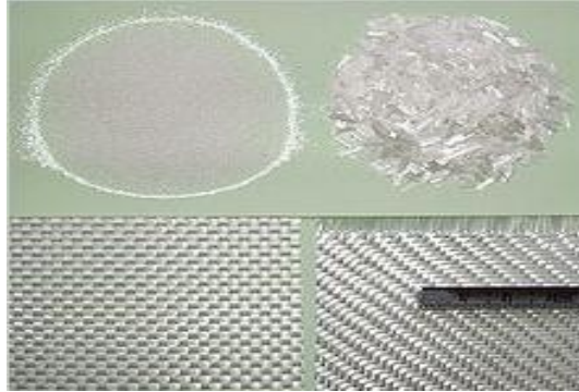
Figure 2: Different physical forms supplied of glass reinforcements; fine ground, chopped, woven ( reference from http://en.wikipedia.org/wiki/Fiberglass )
