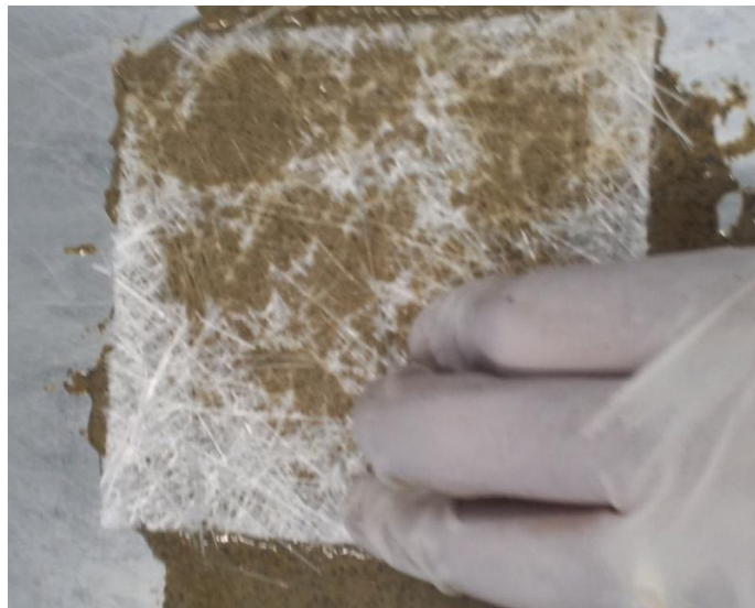
Figure 13: Impregnation method to prepare the fire retardant glass-fiber samples
