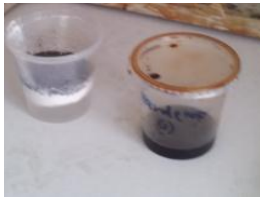
Figure 11: EG was added into the mixed ingredients of APP, BA, and Alumina
