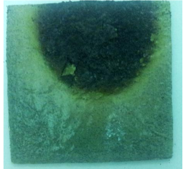
Figure 35: After Fire Test (back)
