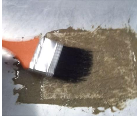
Figure 14: During hand lay-up process
