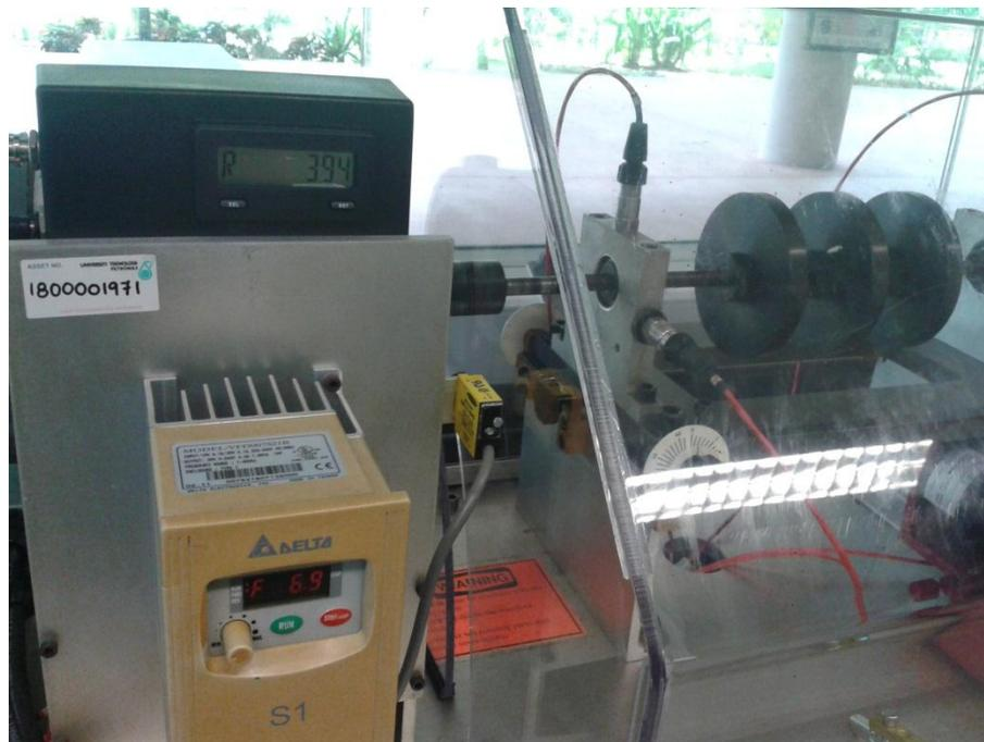
Figure A-4. Speed or frequency controller
