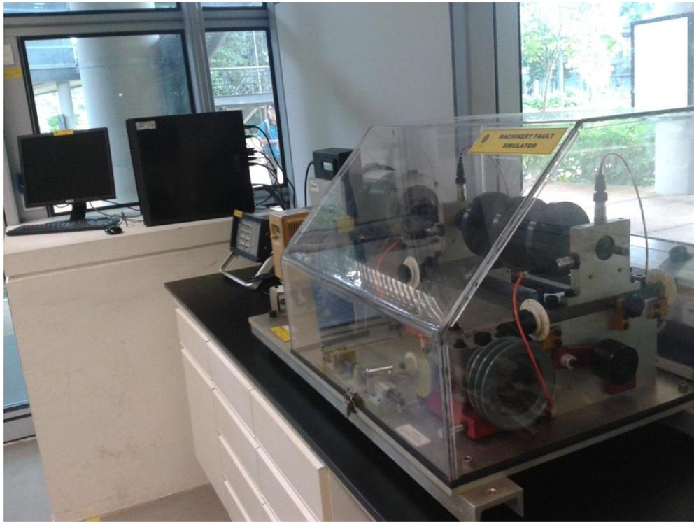
Figure A-5. Overall view of the system (machine fault simulator and the computer that run the LabVIEW software)
