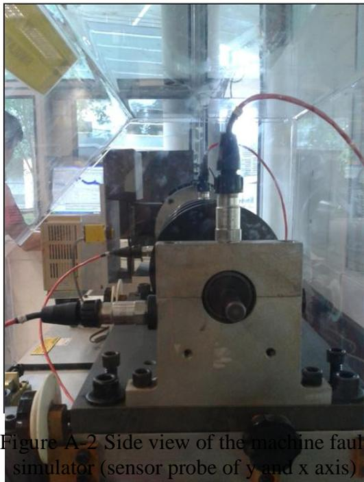
Figure A-2 Side view of the machine fault simulator (sensor probe of y and x axis)
