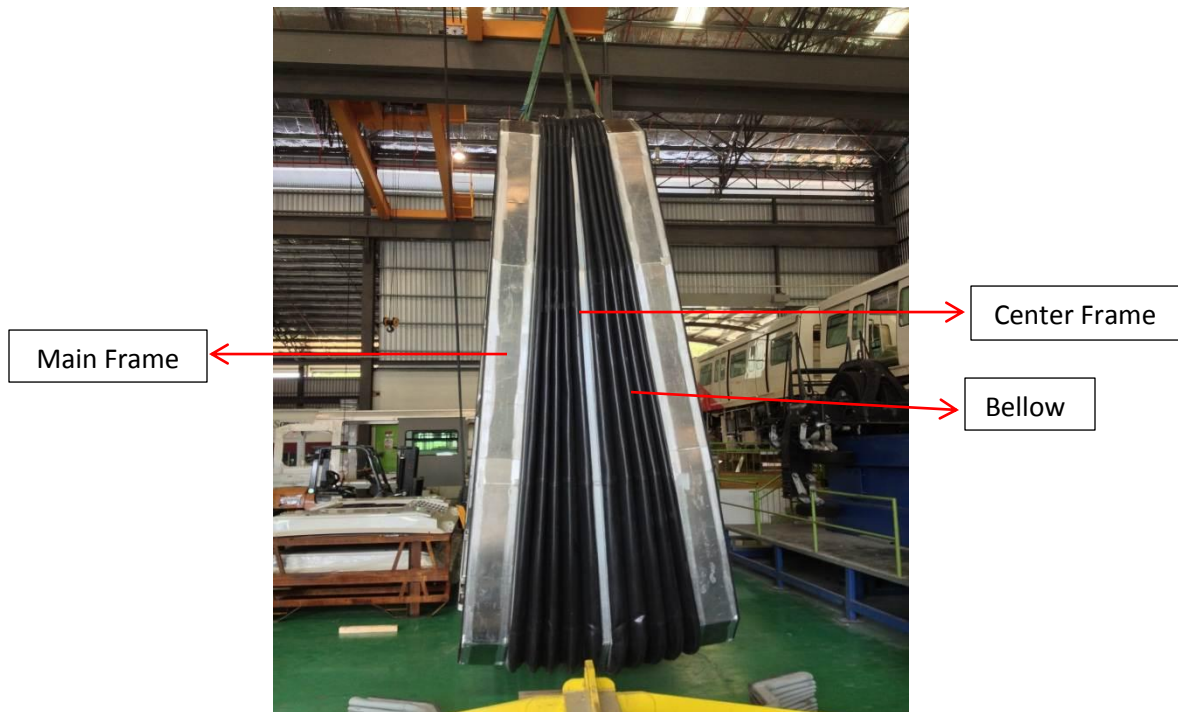
Figure 3: Overweight gangway (SCOMI, 2013)
