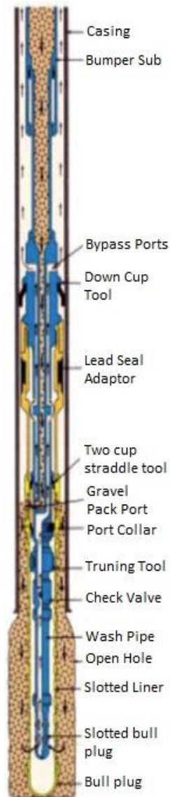
Figure 2.13: Mechanical set cup-type packer (Courtesy of Schlumberger)
