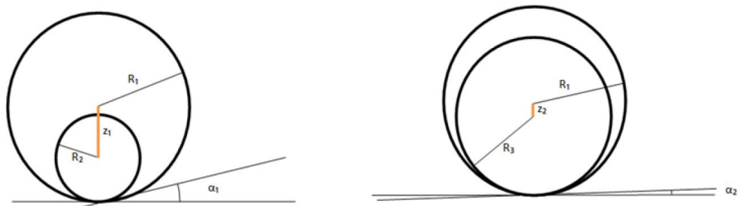
Figure 2.8: Casing Drilling & conventional drilling pipe geometry (Karimi et al., 2011)
