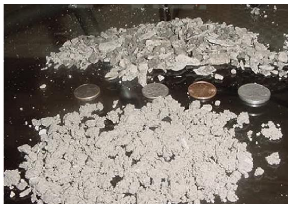
Figure 2.4: Fine Cuttings at Shaker in CwD Application (Tessari, 2009)
