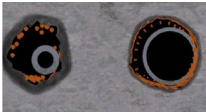
Figure 2.9: Eccentricity of CwD and conventional drilling. (Moellendick & Karimi, 2011)
