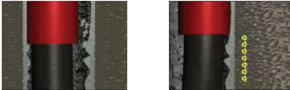
Figure 2.3: Casing is force against bore wall, smearing mud cake and sealing porous formations by producing thinner mud cake. (Moellendick & Karimi, 2011)
