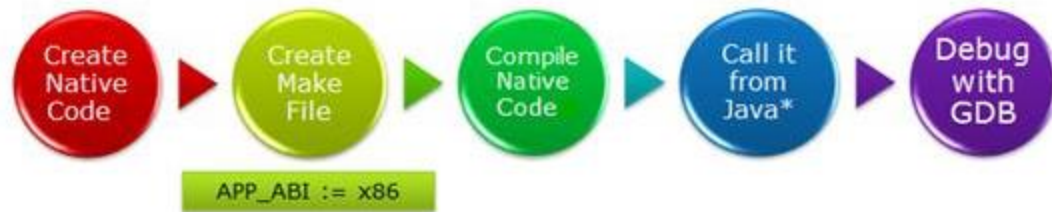
Figure 19: NDK Application Development Process
