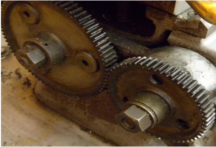
Figure 1.3: Example of Spur Gears Application: Lathe Machine
