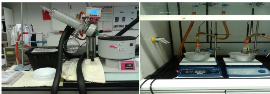
Figure 9: Rotary evaporator and vacuum line
