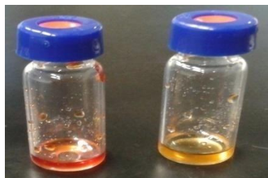
Figure 20: 1-Ethyltetrahydrothiophenium thiocyanate and 1-Ethyltetrahydrothiophenium dicyanamide
