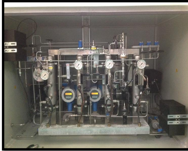
Figure C. 1: Inside view of permeation equipment (CO 2 SMU)
