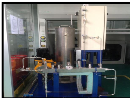
Figure C. 2: Outside view of gas permeation equipment (CO 2 SMU)
