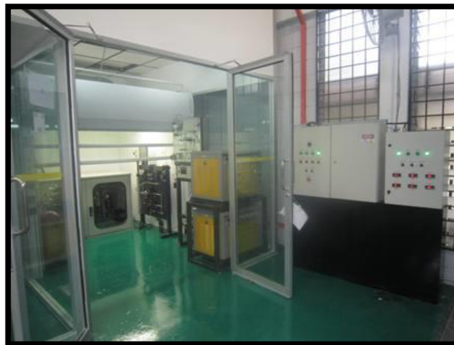
Figure C. 2: Outside view of gas permeation equipment (CO 2 SMU)
