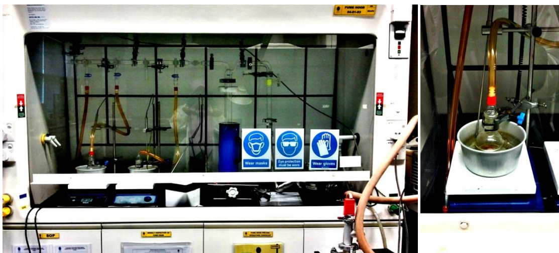
Figure 3.4: Drying the synthesized ILs by using vacuum line for at least 72 hours
