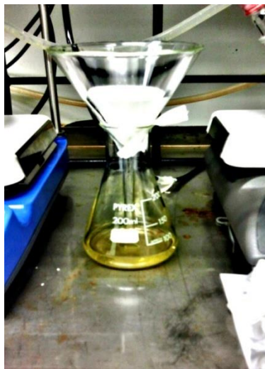
Figure 3.2: Filtration of potassium carbonate from synthesized ILs
