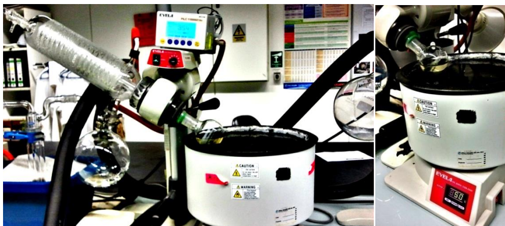
Figure 3.3: Removing any solvents left in synthesized ILs by using rotary evaporator for 2-3 hours
