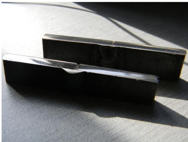
Figure 3.12: Smooth and mirror surface finish of samples.
