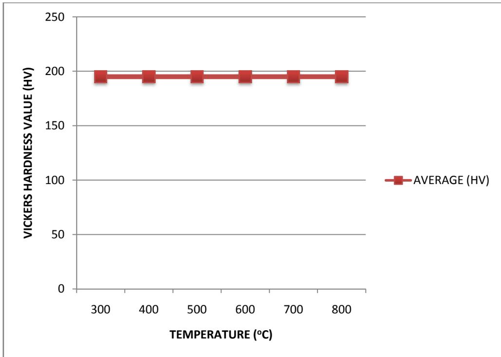
Figure 4.3: Microhardness profile of the weld joints at the position of b-c area.
