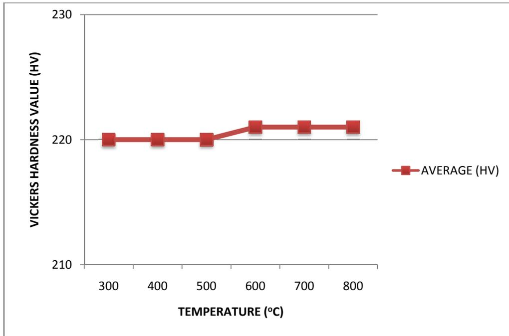
Figure 4.5: Microhardness profile of the weld joints at the position of d-A area.
