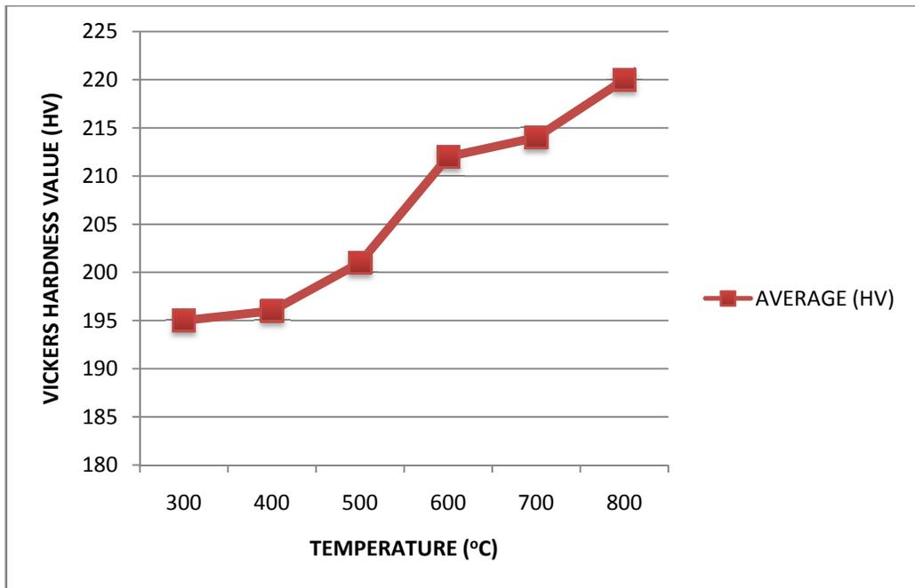
Figure 4.4: Microhardness profile of the weld joints at the position of c-d area.
