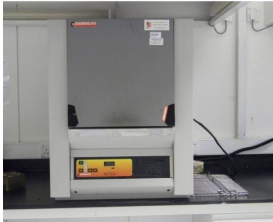
Figure 3.10: Carbolite RHF 1400 used for heat treatment process.
