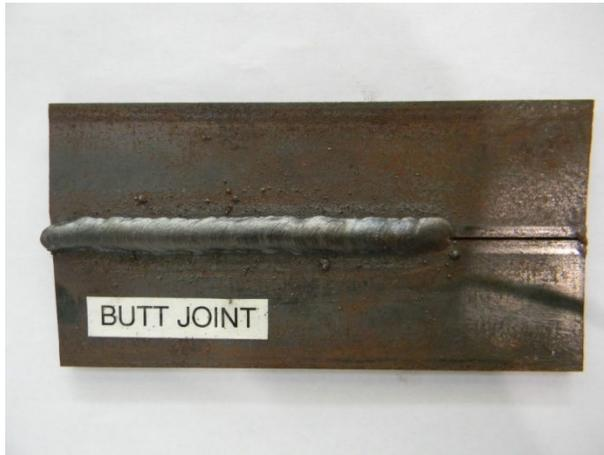
Figure 3.5: Single V butt joint weld.
