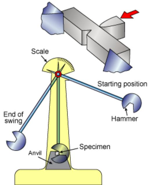
Figure 2.4: Schematic of Charpy test [3].
