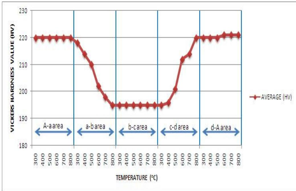
Figure 4.6: Microhardness profile of the weld joints for entire area.
