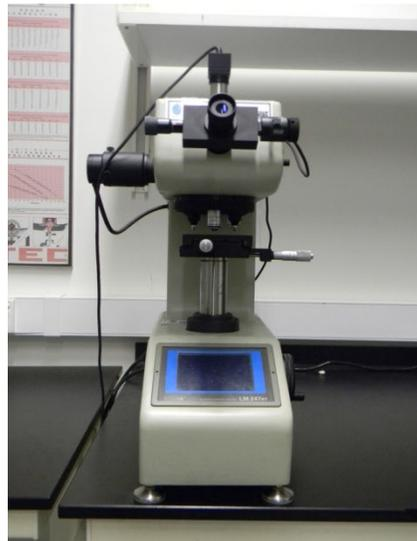
Figure 3.13: Vickers hardness test equipment.
