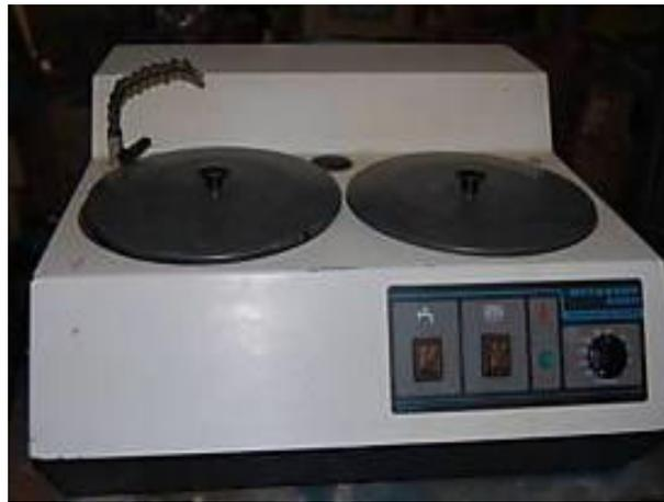
Figure 3.11: Buehler Metaserv 2000 dual polisher grinder.
