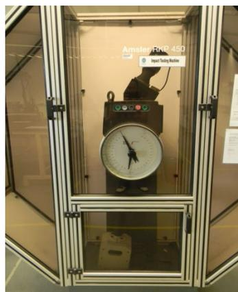
Figure 3.14: Amsler RKP 450 impact testing machine.
