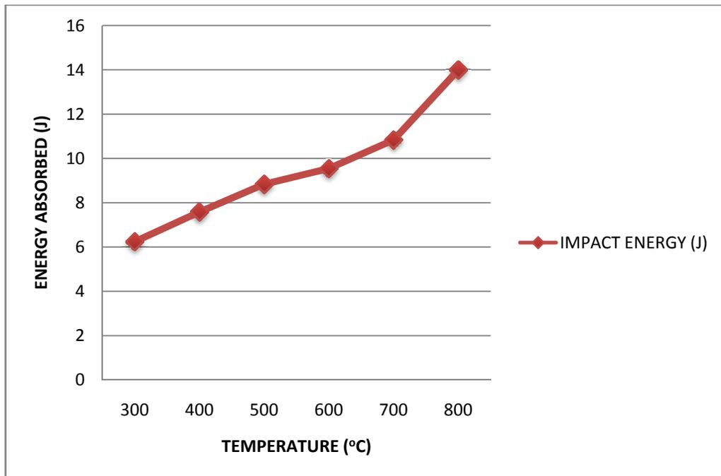
Figure 4.7: Impact energy of HAZ region in various heat temperatures.
