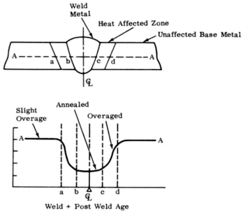
Figure 2.2: Schematic diagram of hardness traverses of welds in each area.
