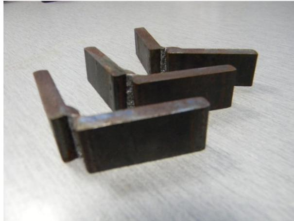
Figure 4.8: Samples structure after impact test.
