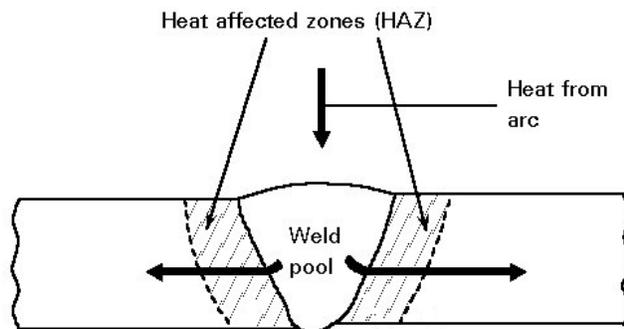
Figure 1.1: HAZ regions in welded joint process [2].
