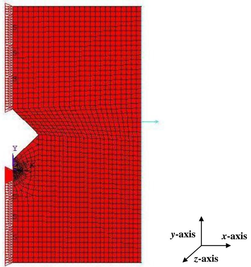
Figure 3.3: ANSYS Model for Mode I Loading of Uniform Tension in  $x$ -axis
