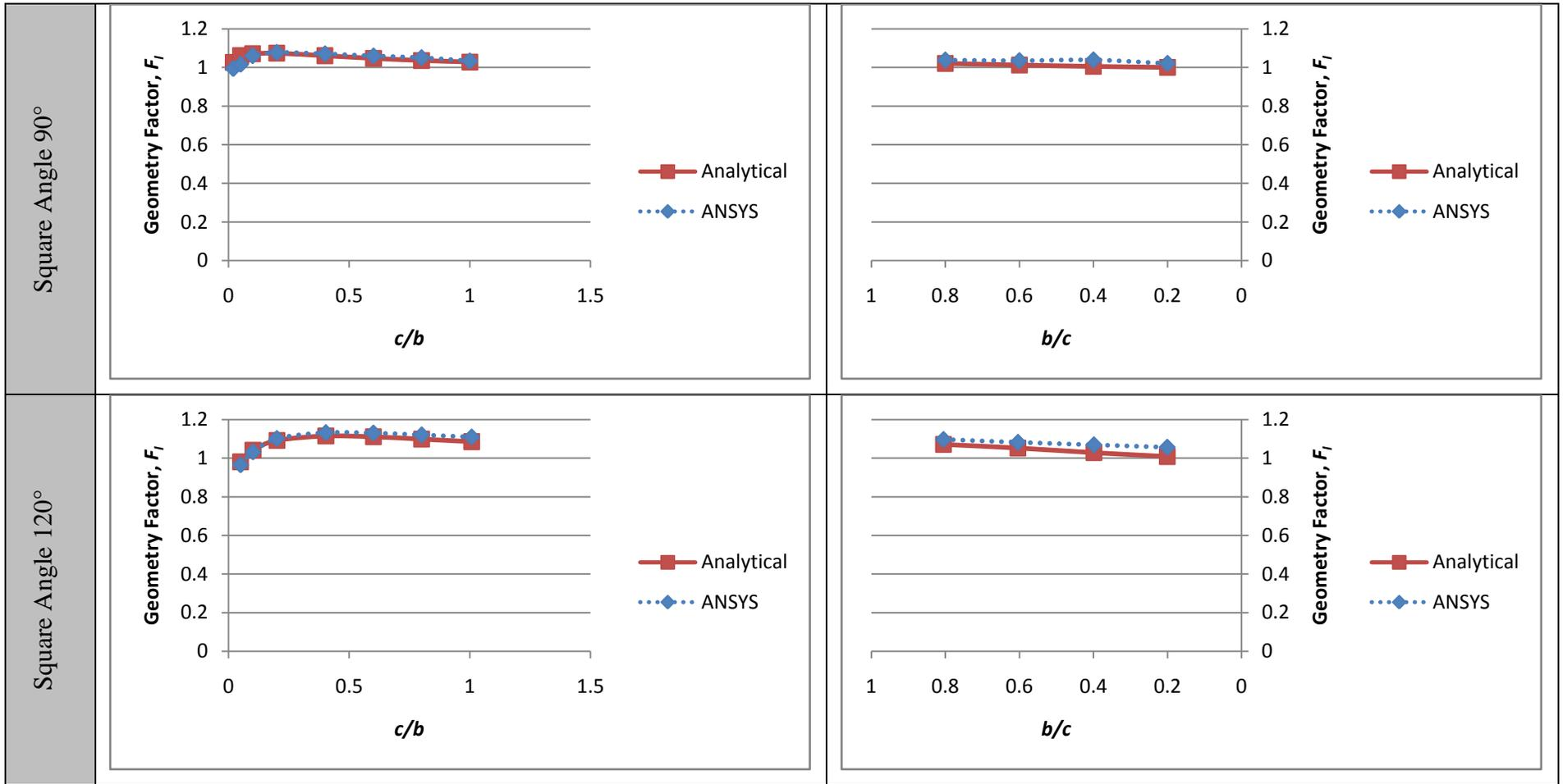
Figure 4.1: Graphical Comparisons of Results for Mode I Loading of Uniform Tension in  $x$ -axis
