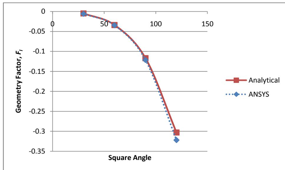
Figure 4.5: Variation of Geometry Factor,  $F$  with Square Angles ( $y$ -axis loading)
