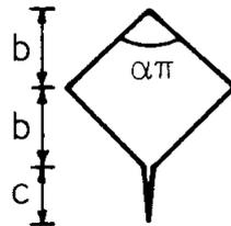
Figure 2.2: A Crack Emanating from the Corner of a Square Hole
