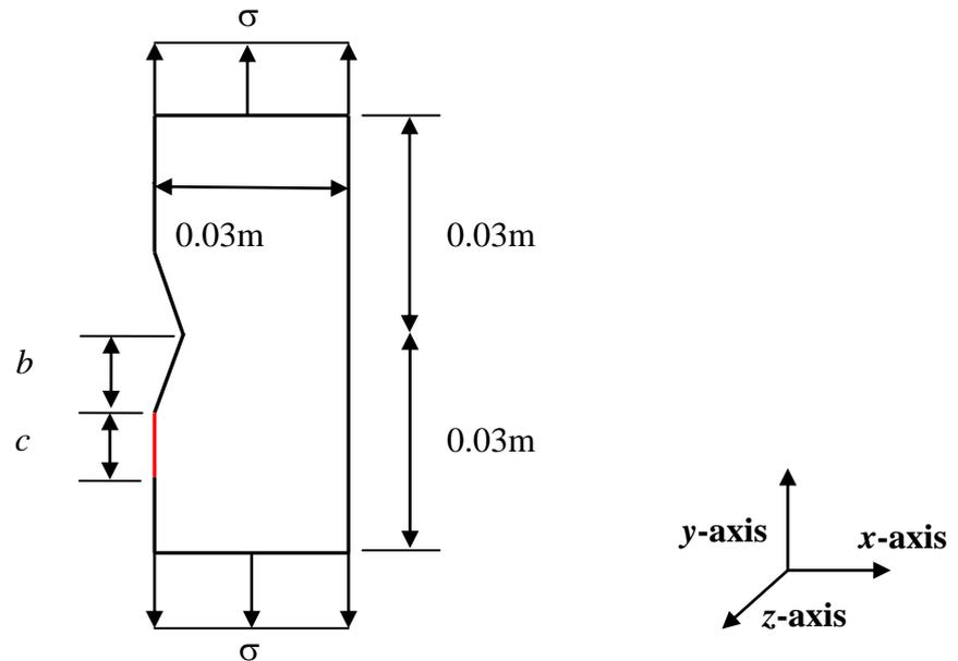
Figure 3.4: Half Model of Crack Geometry in ANSYS with Load Applied in y-axis
