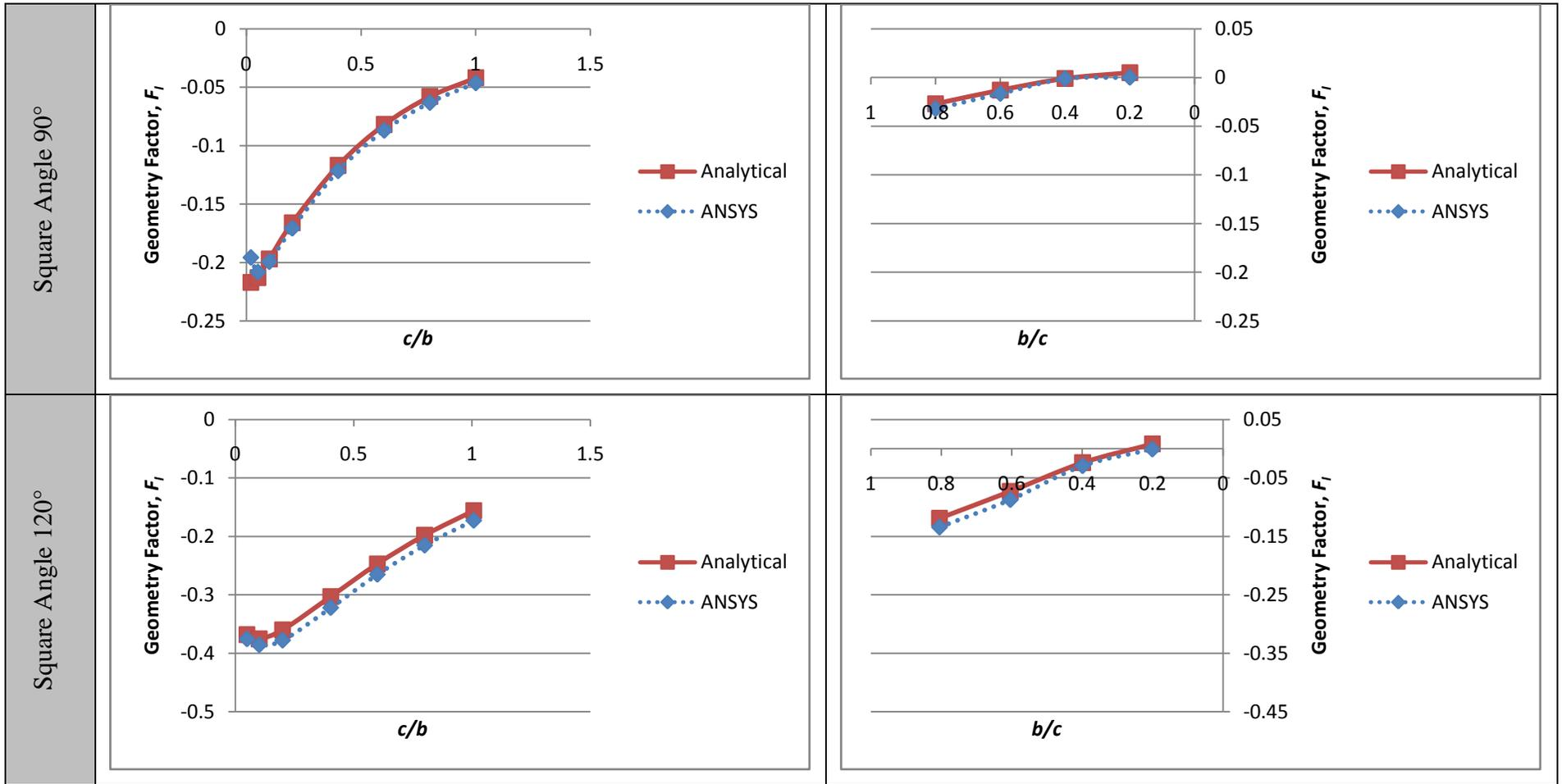
Figure 4.2: Graphical Comparisons of Results for Mode I Loading of Uniform Tension in y-axis
