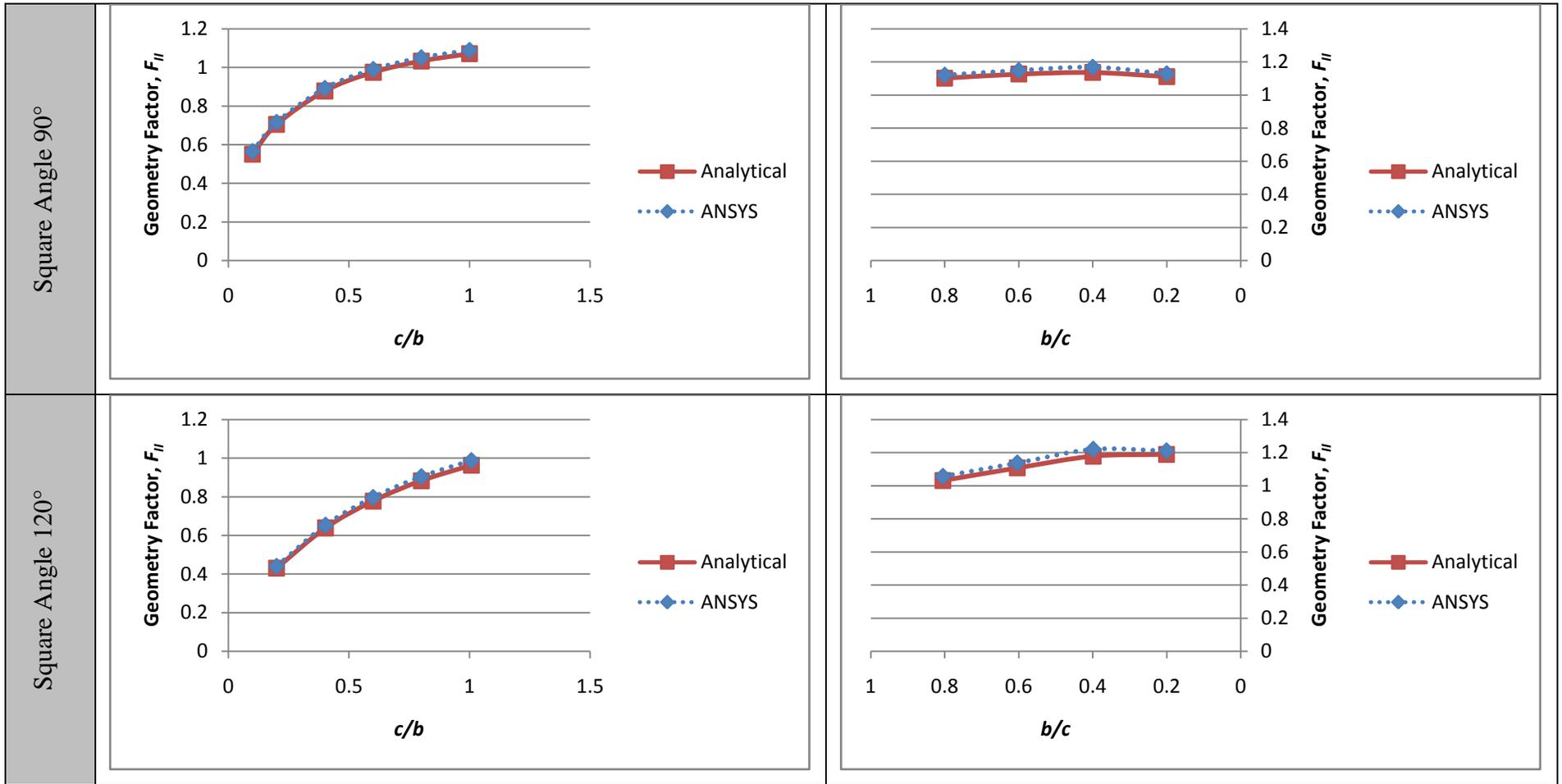
Figure 4.5: Graphical Comparisons of Results for Mode II Loading
