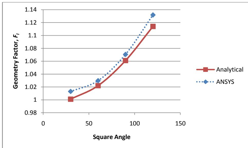
Figure 4.4: Variation of Geometry Factor,  $F$  with Square Angles ( $x$ -axis loading)
