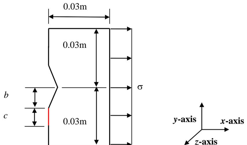
Figure 3.2: Half Model of Crack Geometry in ANSYS with Load Applied in  $x$ -axis
