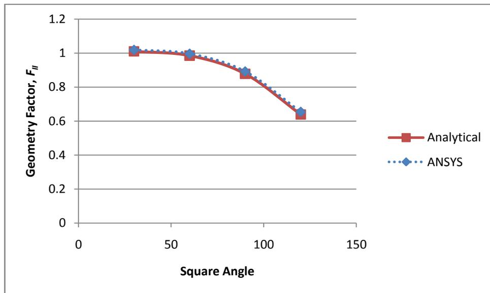
Figure 4.6: Variation of Geometry Factor,  $F$  with Square Angles for Mode II Loading
