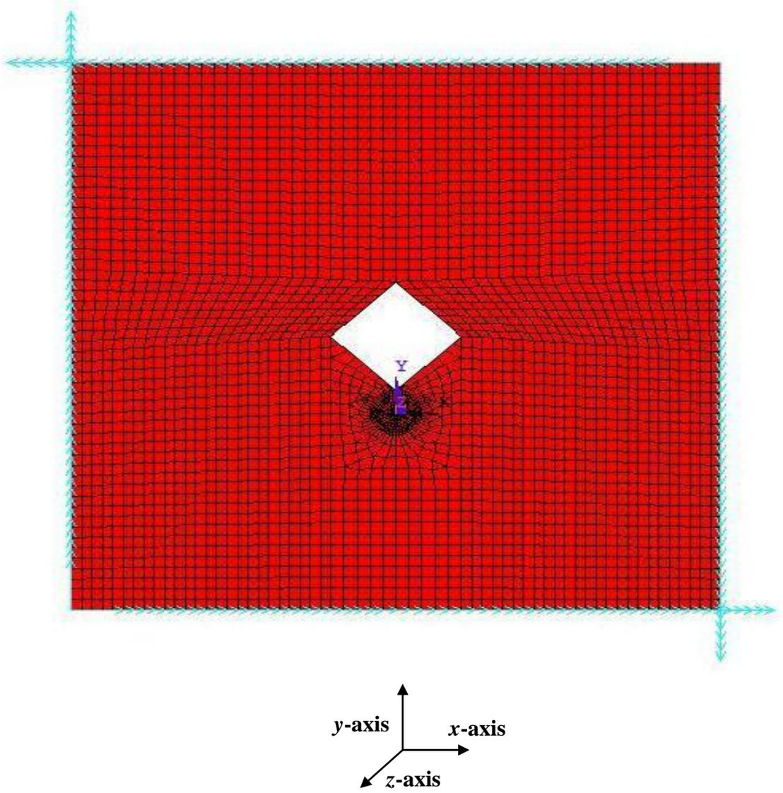
Figure 3.7: ANSYS Model for Mode II Loading
