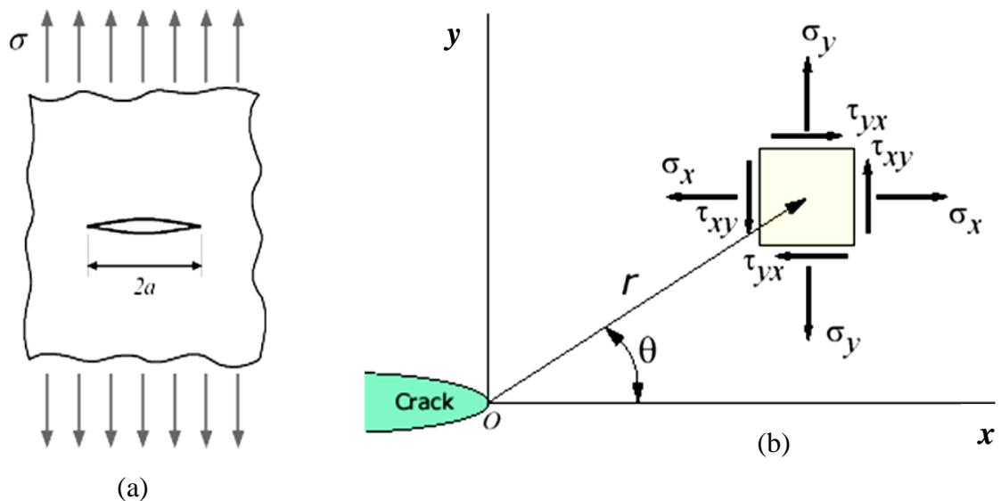
Figure 2.1: (a) A Plate with Uniform Tension in y-axis (b) Normal and Shear Stress Components of an Element around the Crack Tip in a Plate
