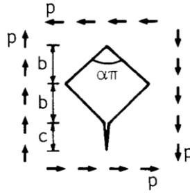
Figure 2.2: A Crack Emanating from a Corner of a Square Hole for Mode II Loading
