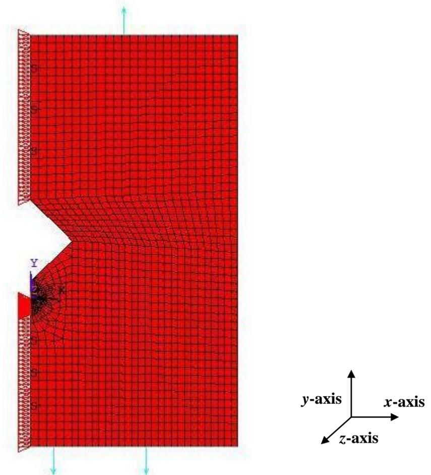
Figure 3.5: ANSYS Model for Mode I Loading of Uniform Tension in y-axis
