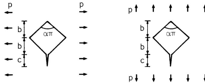
Figure 2.1: A Crack Emanating from a Corner of a Square Hole for Mode I Loading
