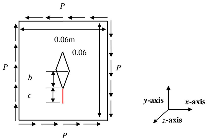
Figure 3.6: Full Model of Cracked-Geometry in ANSYS with Pure Shear Acting along the Geometry Surface
