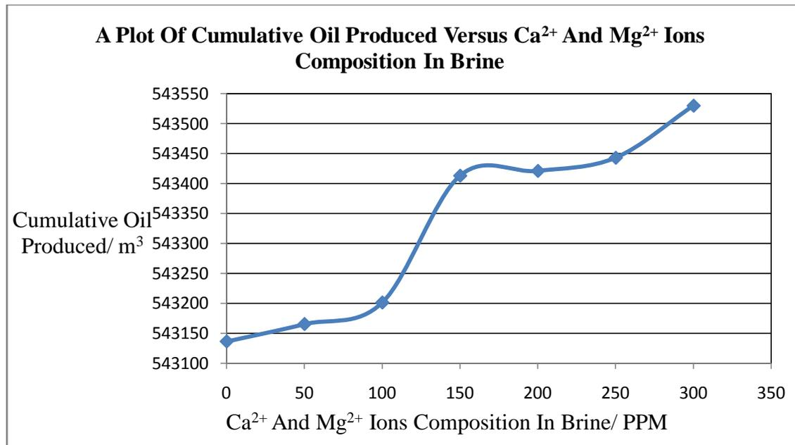
Figure 9- A Plot Of Cumulative Oil Produced Versus Ca<sup>2+</sup> & Mg<sup>2+</sup> Ions Composition.
