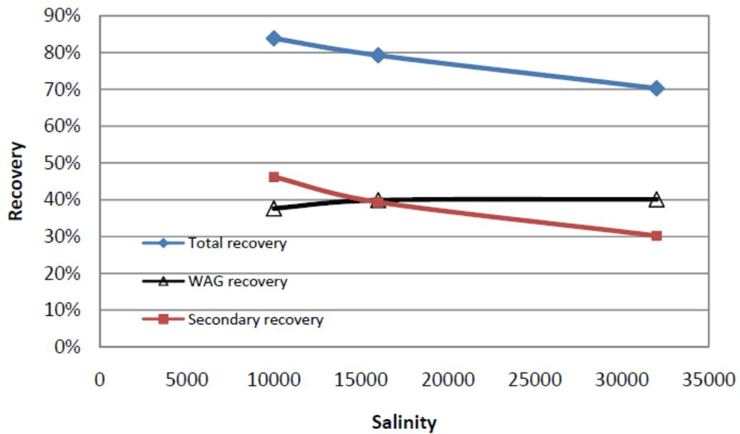
Figure 3:- The recovery of water flooding, WAG flooding and total as a function of salinity.
