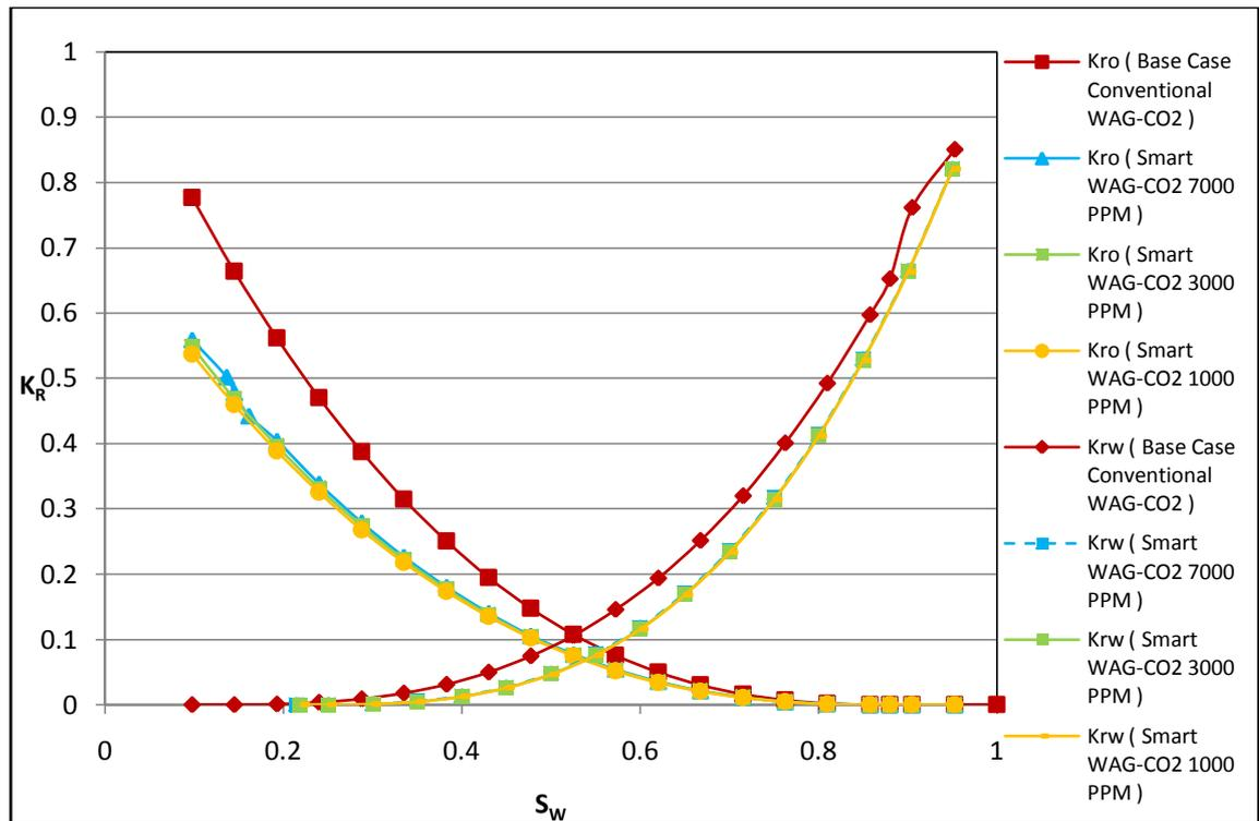
Figure 8:- Relative permeability curves of  $k_{RO}$  and  $k_{RW}$  versus  $S_w$ .
