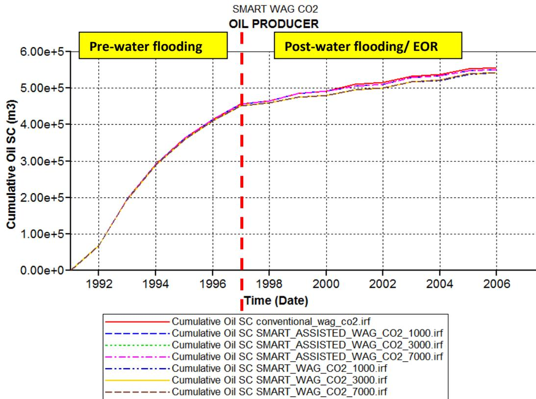
Figure 10:- A Plot Of Cumulative Oil Produced For 7 Different Injection Scenarios.
