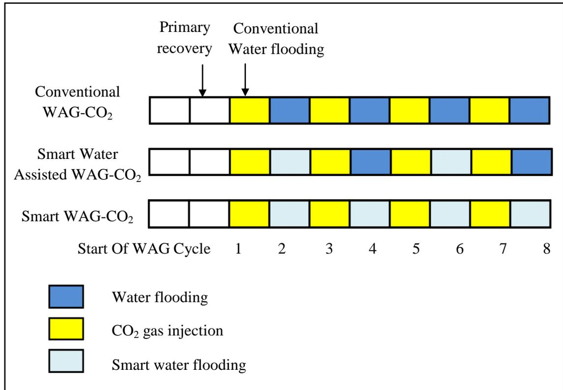
Figure 7:- Simulation design of three different injection scenarios.
