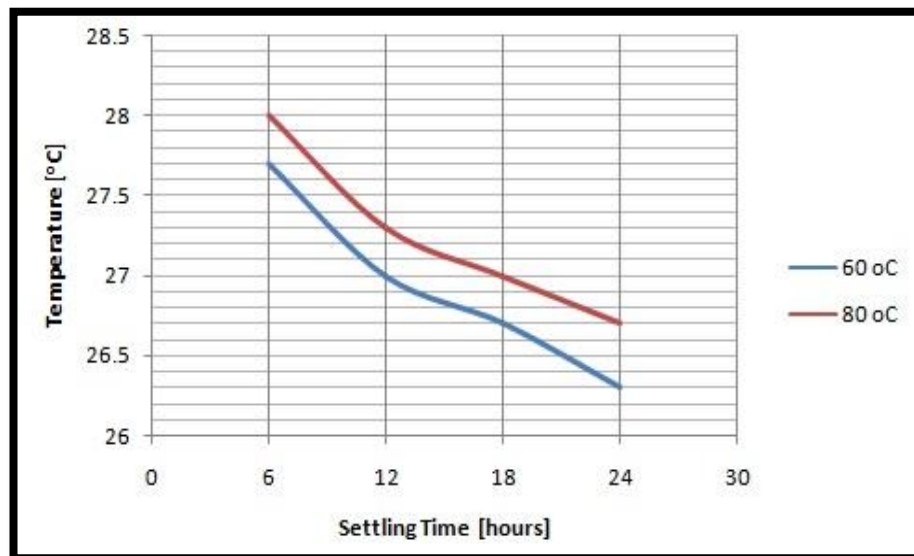
Figure 19: Pour Point Value for Different Settling Time (Tilt Method)
