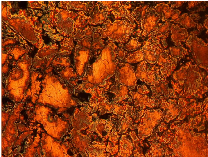
Figure 3.1. Optical micrograph image of cross section of the typical AISI 430 steel.
