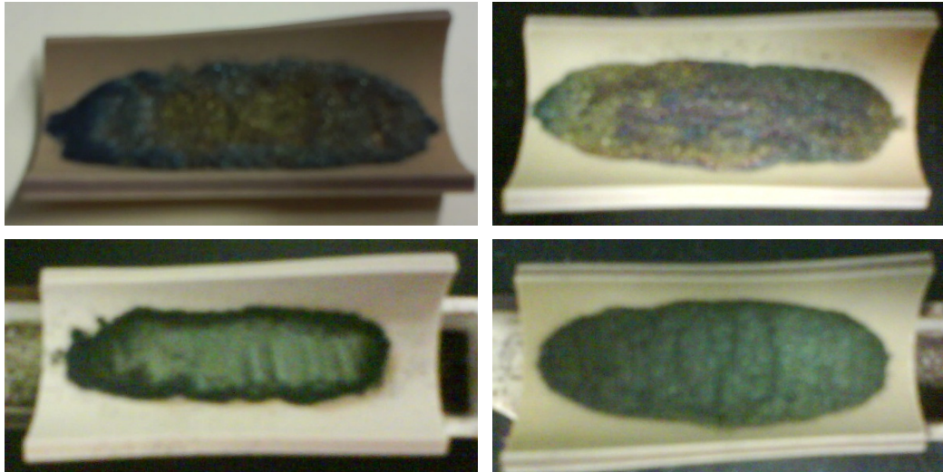
Figure 2.3. Samples of AISI 430 ferritic stainless steel powders after having nitriding process.
