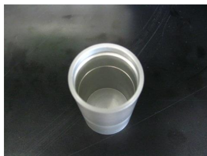
Figure 9e: Test Specimen being transferred into test cup for automatic rotational method
