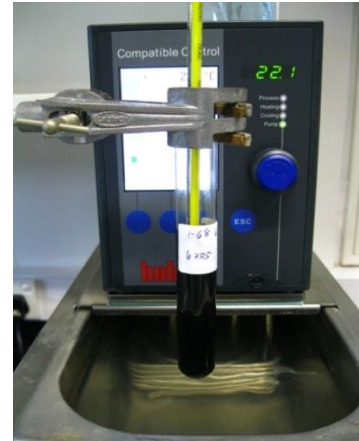
Figure 10b: The specimen is let to cool naturally until temperature reaches 30°C
