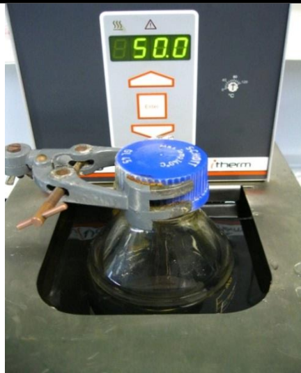
Figure 9a: Sample originally in large bottle being heated up and stirred
