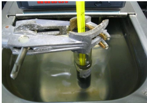
Figure 10c: The Specimen is immersed in water bath set to cool from 30°C to 10°C
