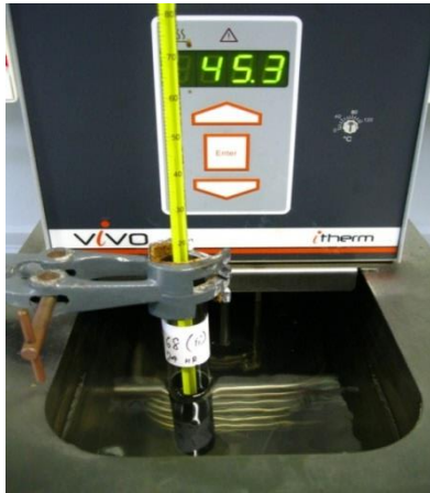
Figure 10a: 2nd preheat process at approximately 45°C inside the hot water bath
