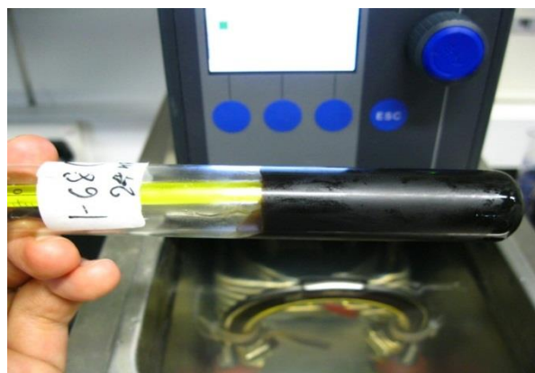
Figure 10d: Final tilt act showing the specimen has ceased to flow for at least 5 seconds.
