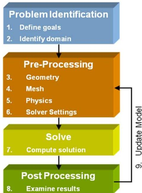
Figure 8 : Flow Chart of CFD Analysis
