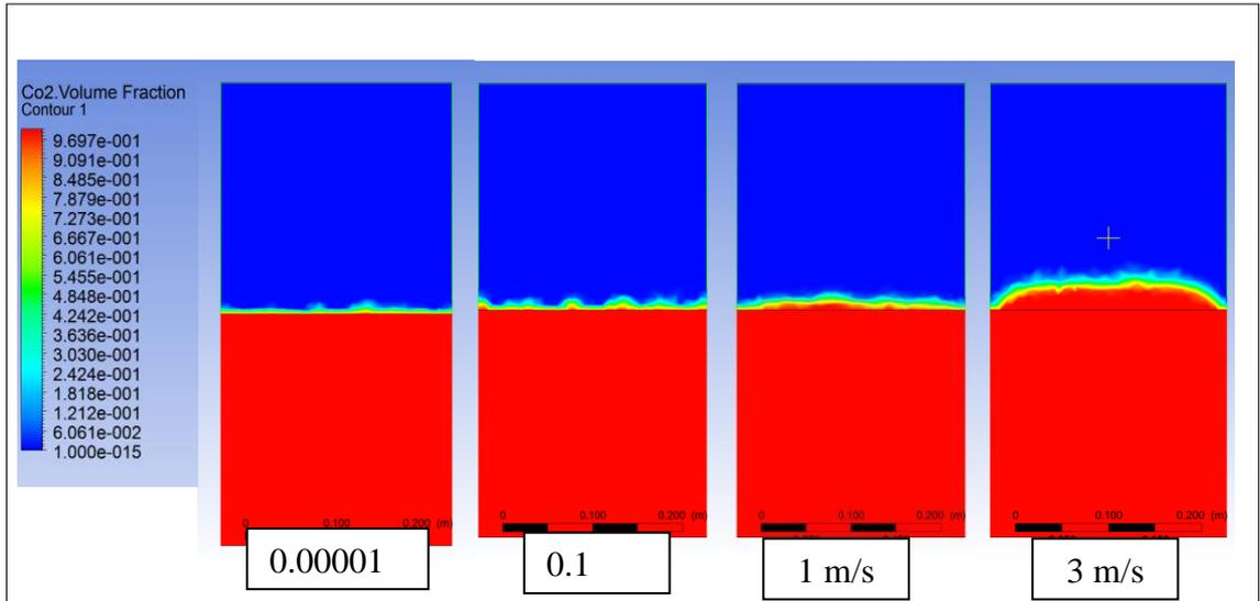
Figure 19: CO<sub>2</sub> Volume Fraction for different inflow velocity
