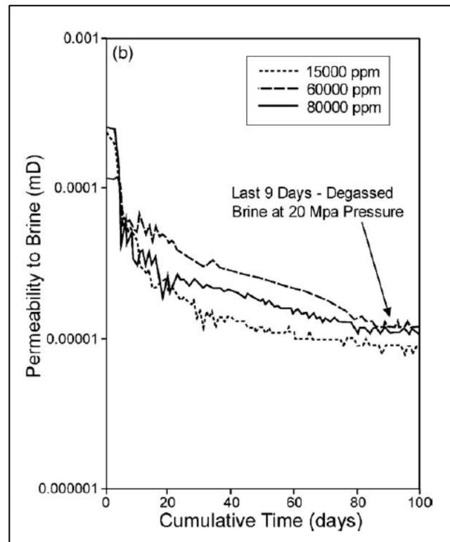
Figure 10: Permeability profile of Portland cement [21]
