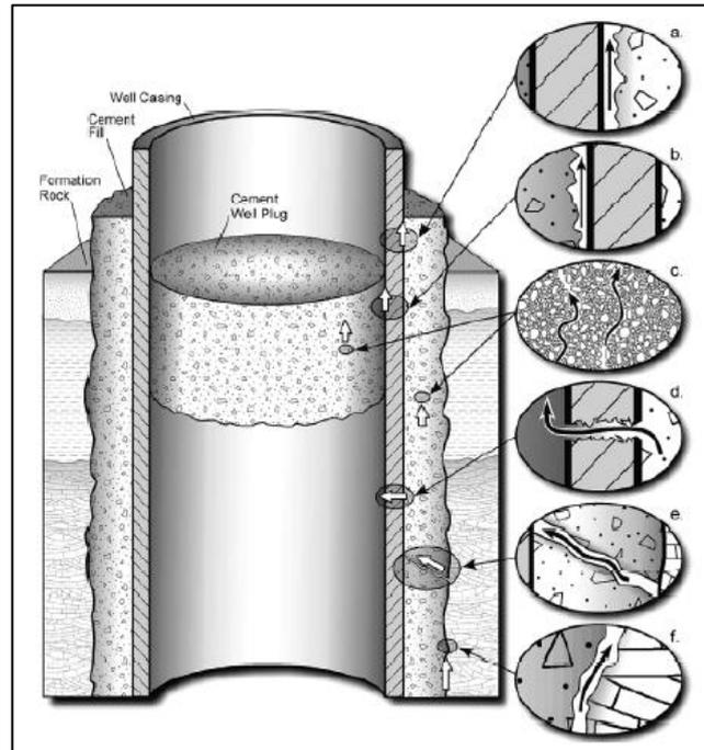
Figure 2: Potential leakage paths for CO<sub>2</sub> in well system a) between outside cement and casing b) between outside cement and casing c) through cement plug steel casing d) through the casing e) through cement or fractured cement f) interface between cement and formation rock [6]
