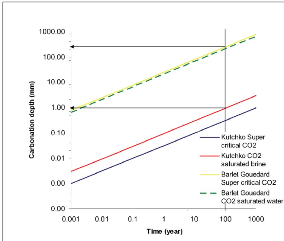
Figure 7: Carbonation depth estimated from laboratory test [5]
