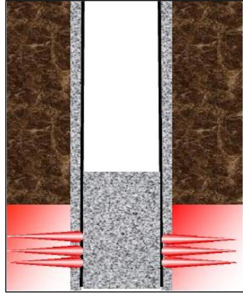
Figure 4: Cement plug set across perforation [18]
