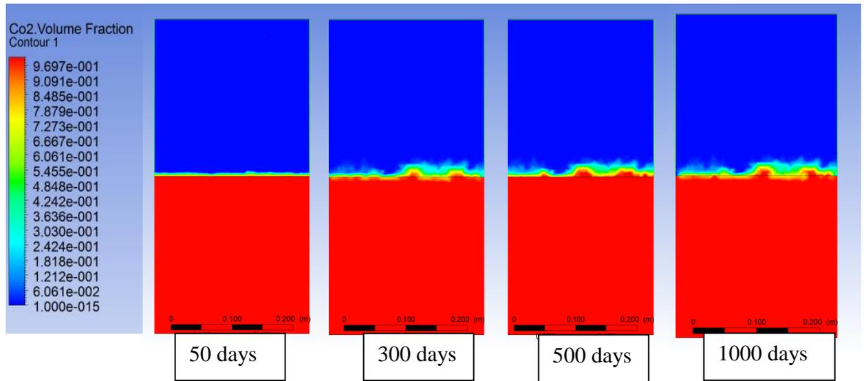
Figure 13: Volume fraction of CO<sub>2</sub> for base case model
