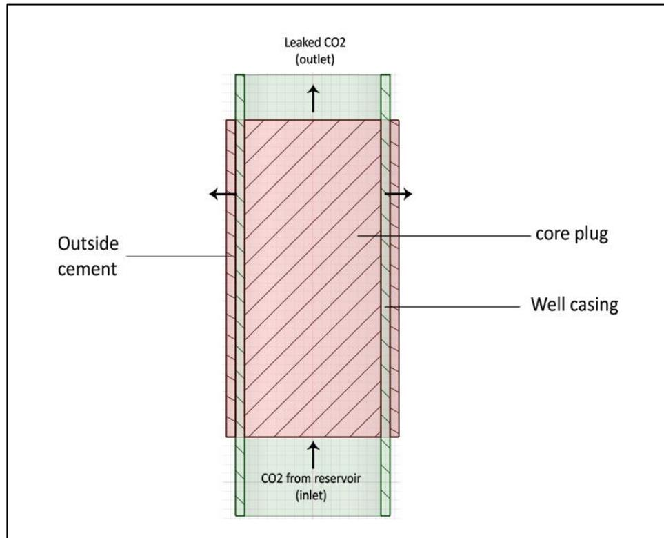
Figure 9: CO<sub>2</sub> Leakage in abandon well geometry model.
