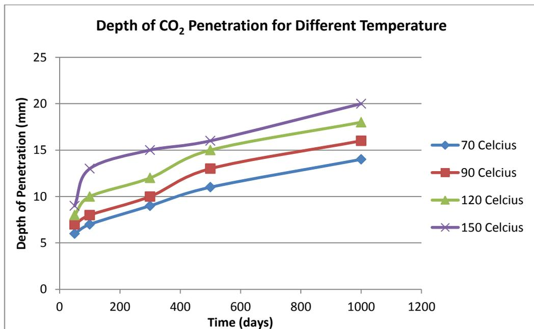
Figure 23: Depth of CO<sub>2</sub> Penetration
