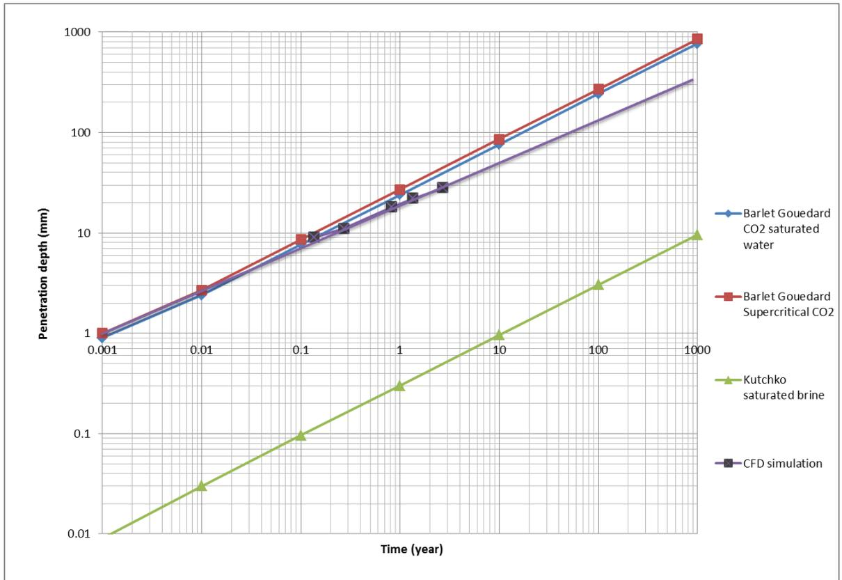
Figure 16: Comparison of CFD run with laboratory data
