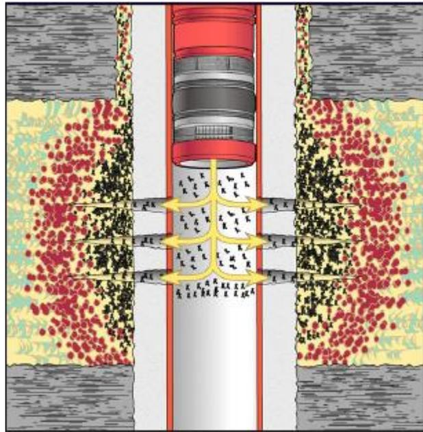
Figure 5: Cement squeeze with retainer into perforation [18]
