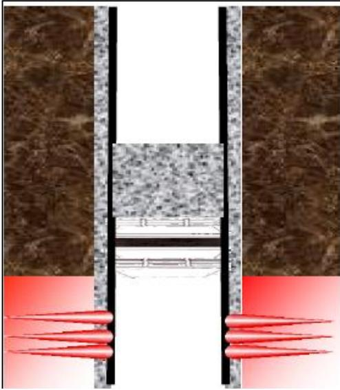
Figure 3: Bridge plug capped with 8 meters of cement [18]
