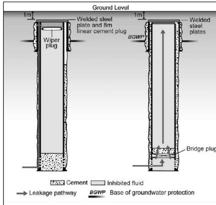
Figure 1: Typical abandonment of cased and completed well [7]
