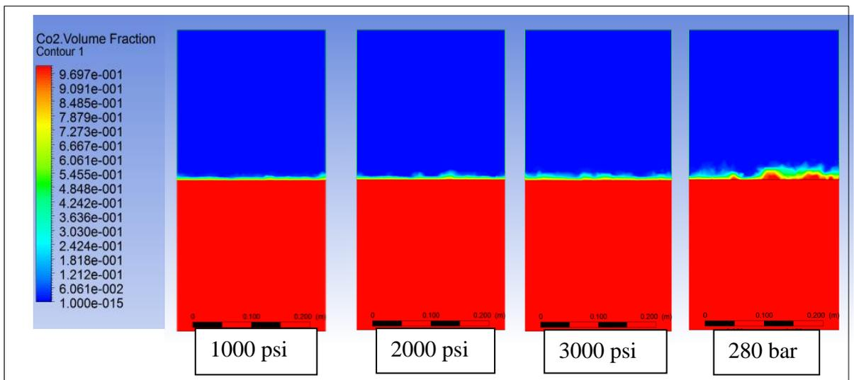
Figure 21: CO<sub>2</sub> Volume Fraction for different pressure
