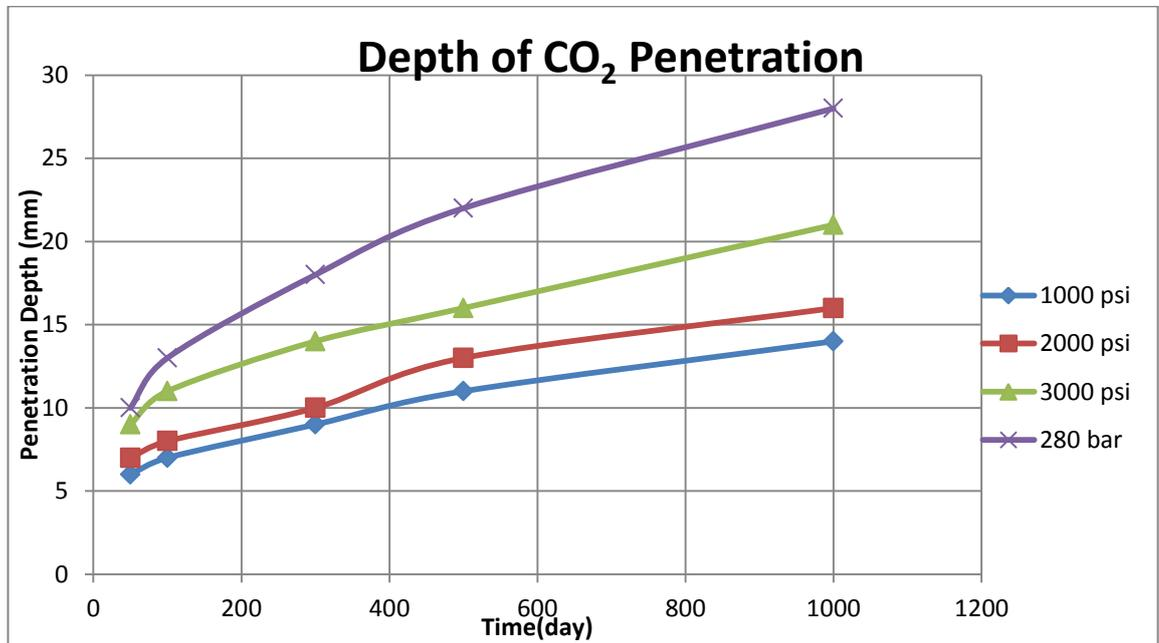
Figure 22: CO<sub>2</sub> Penetration depth for different pressure
