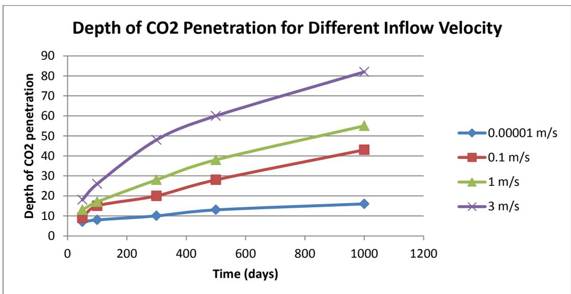
Figure 20: Depth of CO<sub>2</sub> Penetration for different inflow velocity
