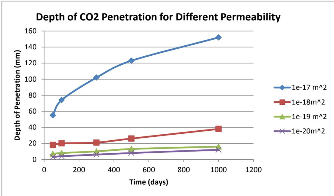
Figure 18: Depth of CO<sub>2</sub> Penetration for Different Permeability
