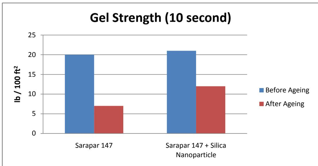
Figure 11: Gel strength (10 second) bar chart for Sarapar 147 and Sarapar 147 + Silica Nanoparticle
