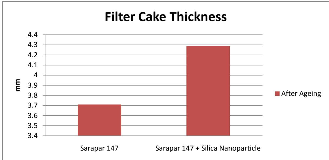
Figure 15: Filter cake thickness bar chart for Sarapar 147 and Sarapar 147 + Silica Nanoparticle
