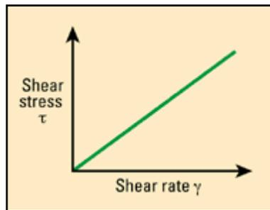
Figure 3: Flow Curve for a Newtonian Fluid<sup>[9]</sup>
