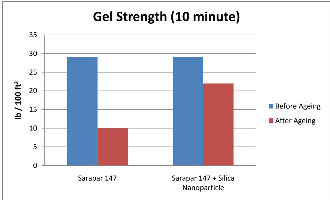
Figure 12: Gel strength (10 minute) bar chart for Sarapar 147 and Sarapar 147 + Silica Nanoparticle
