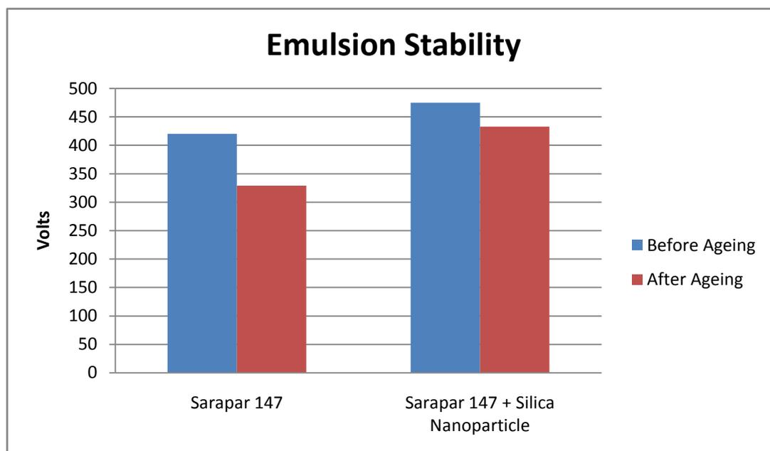
Figure 13: Emulsion stability bar chart for Sarapar 147 and Sarapar 147 + Silica Nanoparticle
