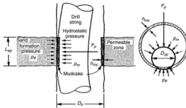
Figure 2: Mechanism of differential sticking problem. <sup>[6]</sup>
