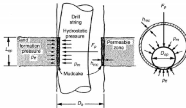
Figure 2: Mechanism of differential sticking problem. [6]
