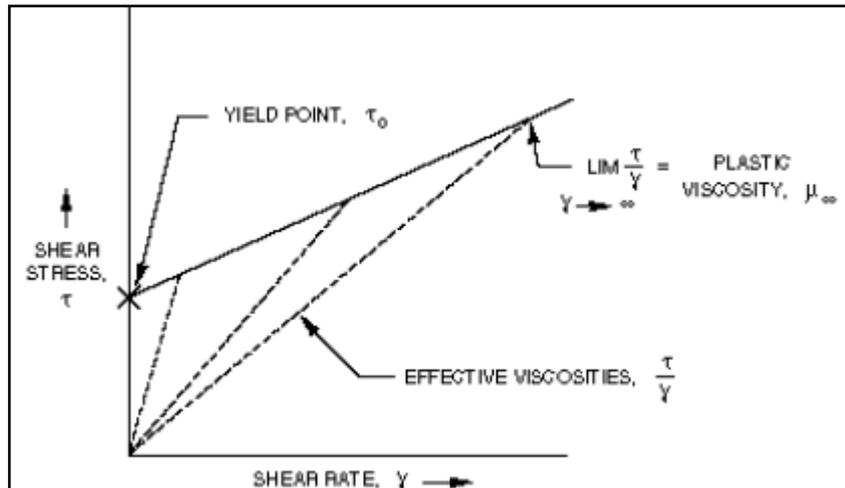
Figure 4: Flow Curve for a Bingham Plastic Fluid [9]
