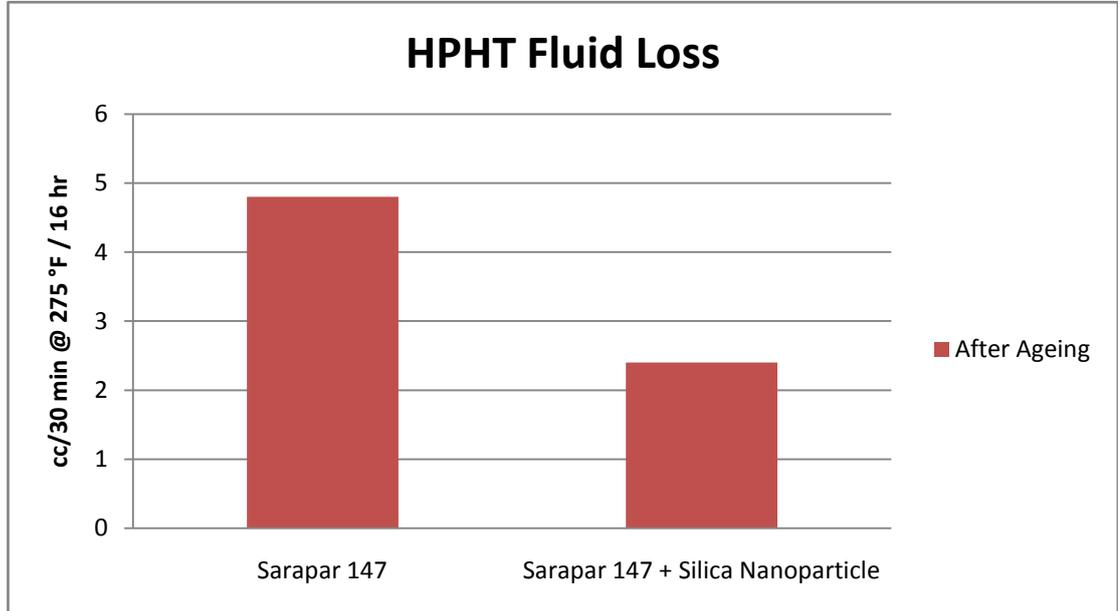
Figure 14: HPHT fluid loss bar chart for Sarapar 147 and Sarapar 147 + Silica Nanoparticle
