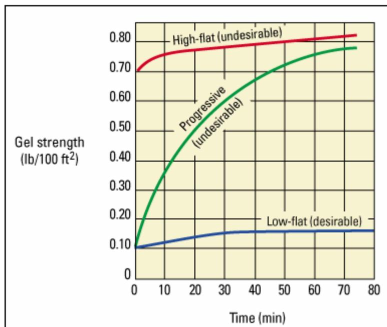
Figure 6: Gel Strength Characteristics vs. Time [9]
