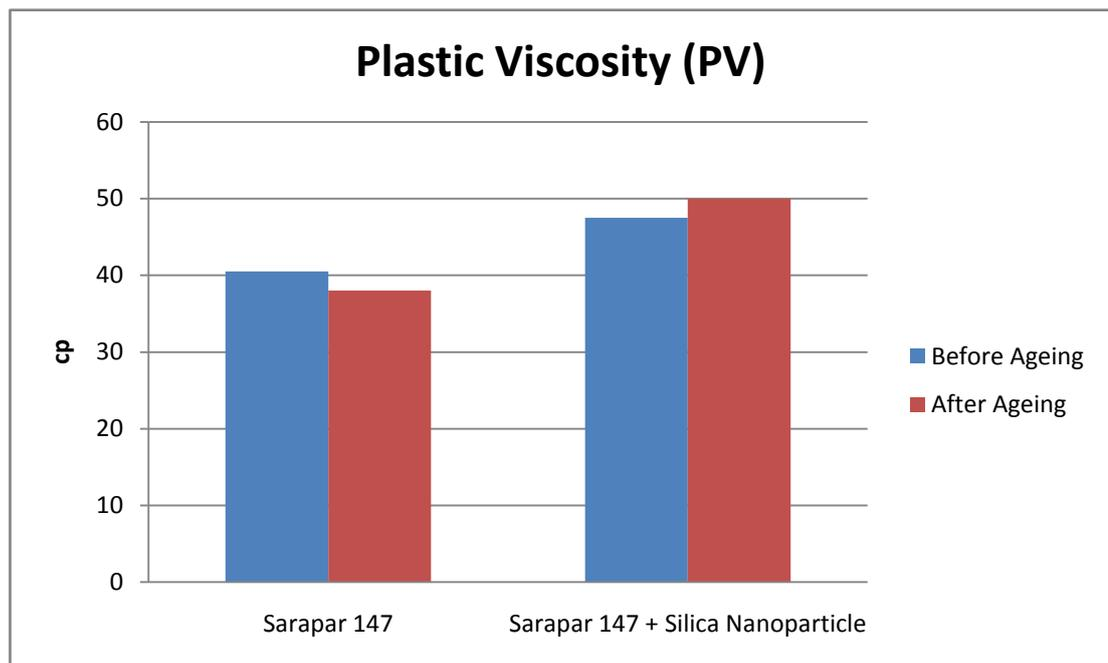
Figure 9: Plastic viscosity bar chart for Sarapar 147 and Sarapar 147 + Silica Nanoparticle
