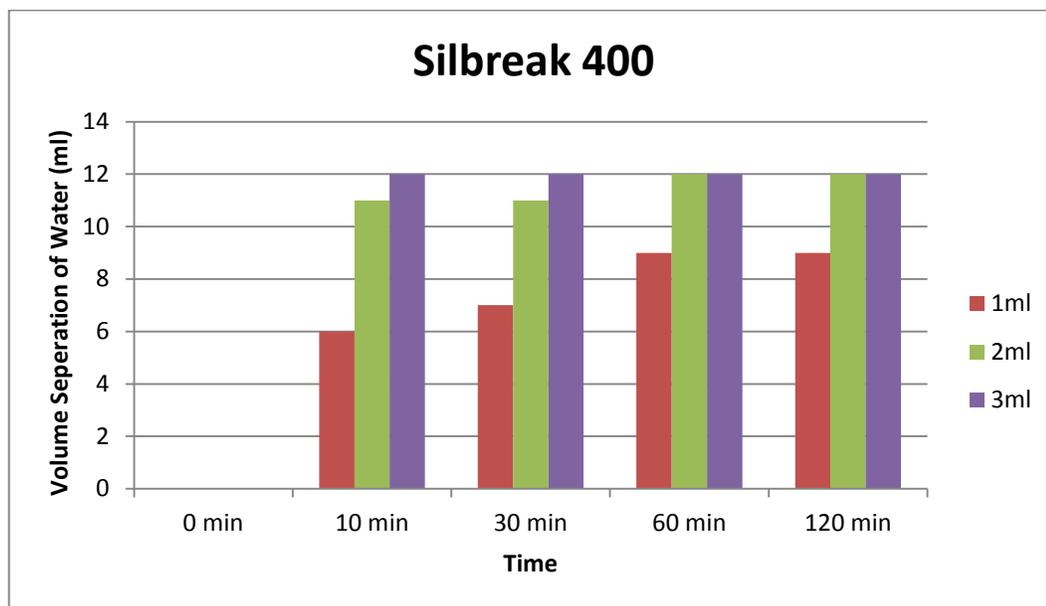
Figure 4.2 : Volume Separation of Water using Sillbreak 400
