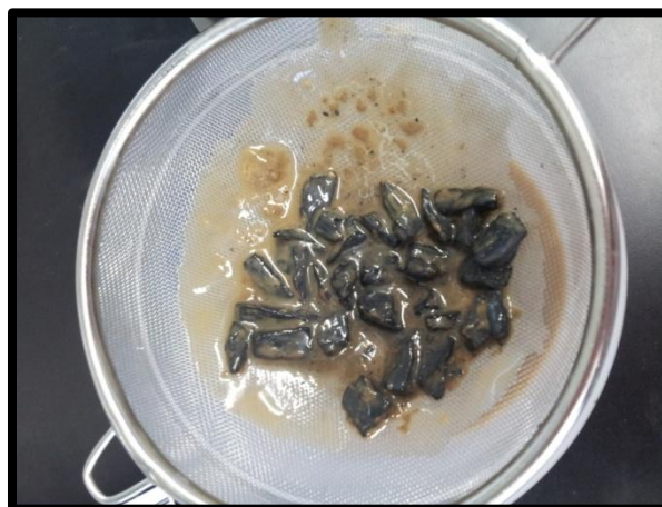
Figure 11 : Undispersed shale after hot rolled
