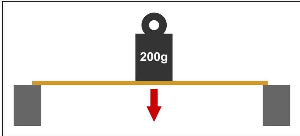
Figure 35: Deflection test configuration
