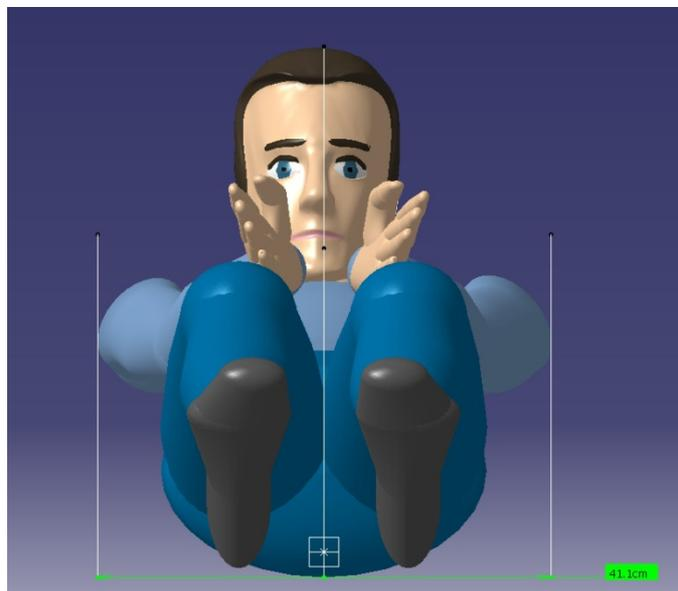
Figure 14: Width of the driver position
