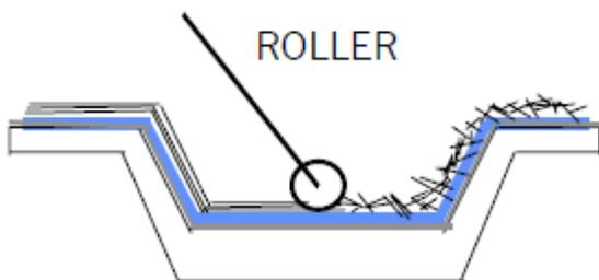
The previous step is repeated so that another layer is applied to get a two layer reinforced composite.
