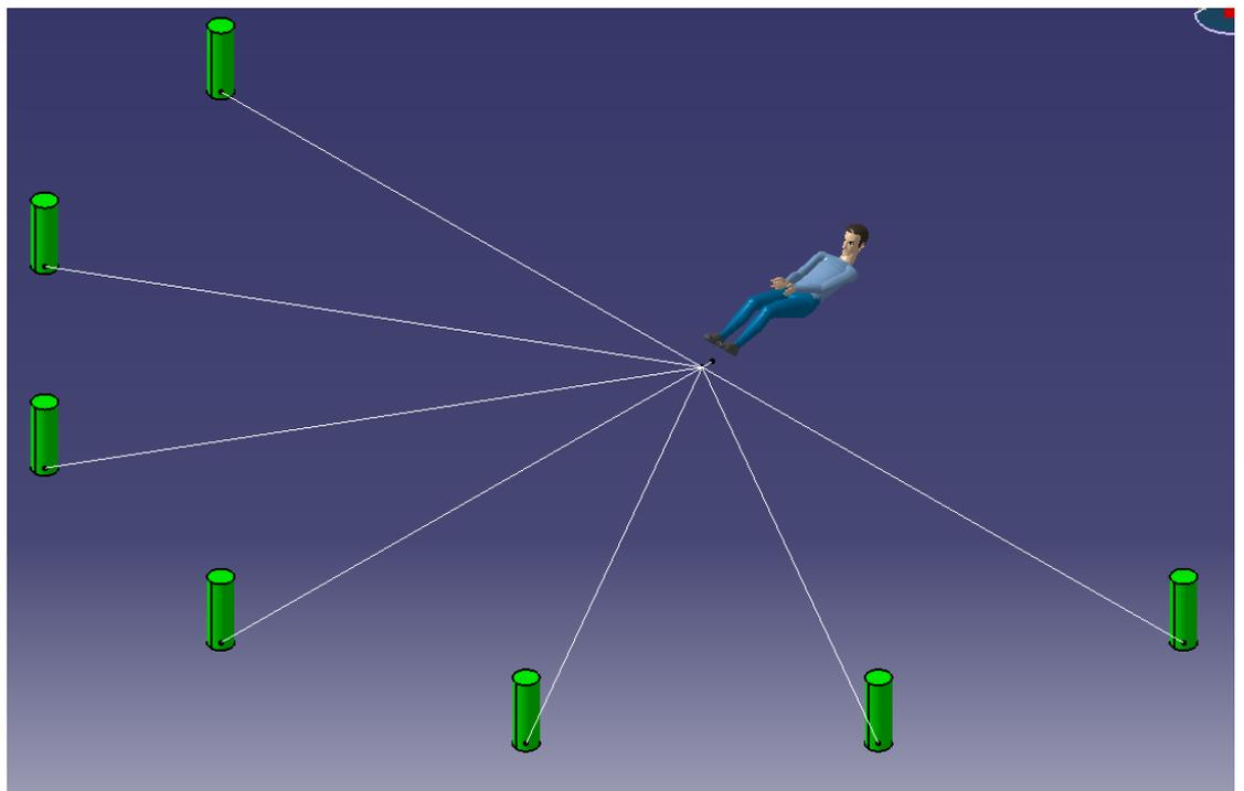
Figure 15: Visibility assessment layout with driver in position
