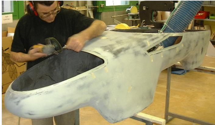
Figure 10: Monocoque of the Pac-Car II.
