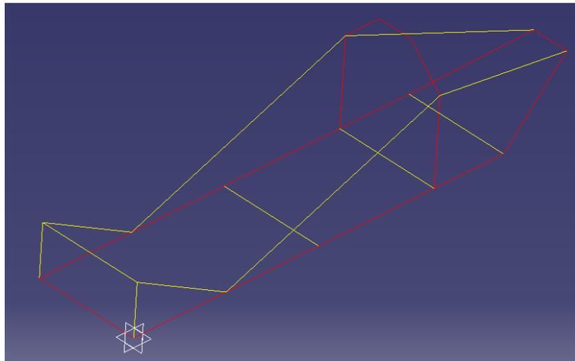
Figure 19: Ladder frame concept design
