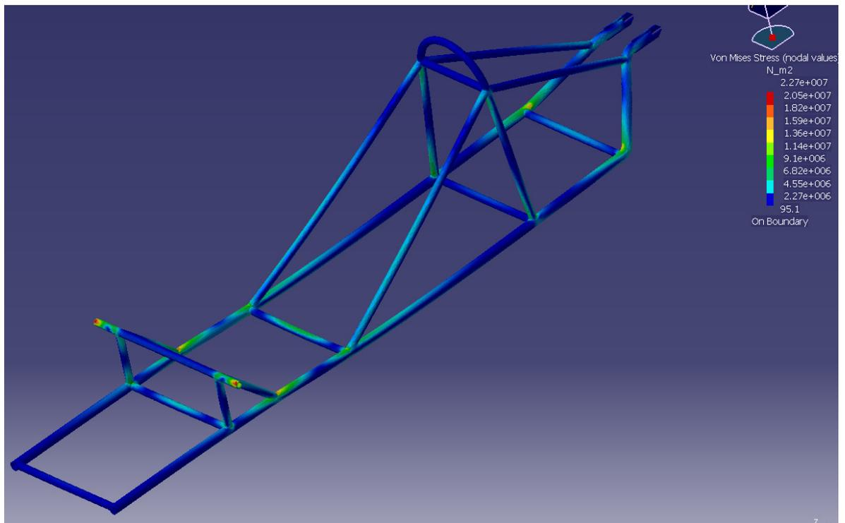
Figure 29: Maximum Von Mises Stress of chassis frame
