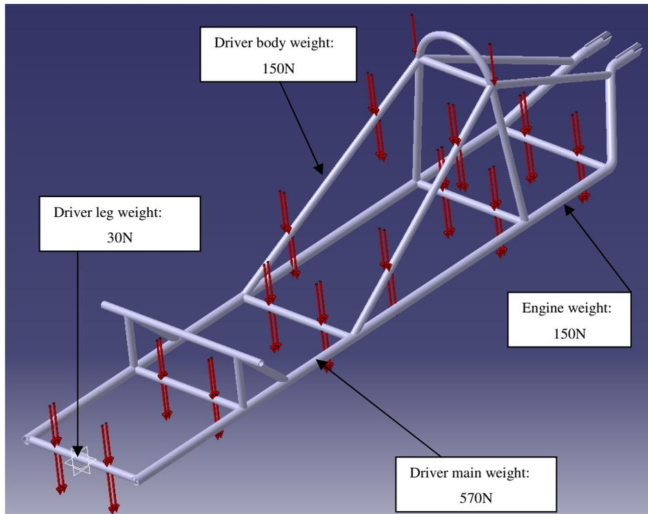
Figure 26: Application of Loads with Safety Factor on the Chassis Frame
