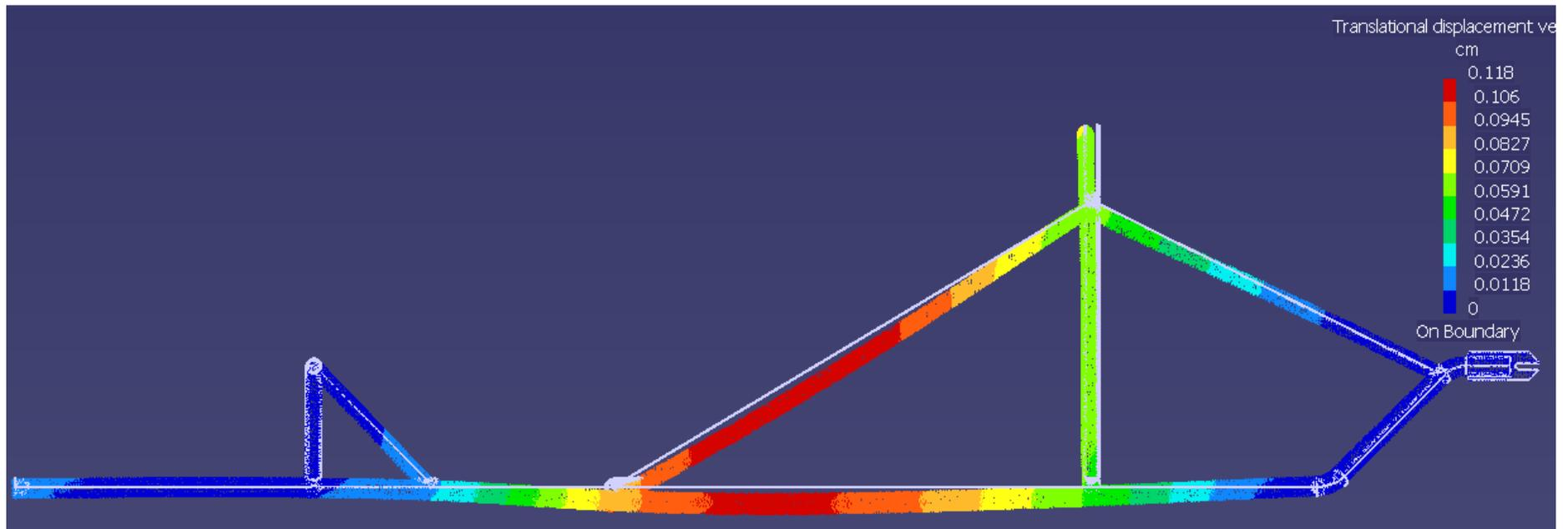
Figure 27: Deflection of the frame with applied static loads with 20 times amplification and comparison to the original shape.
