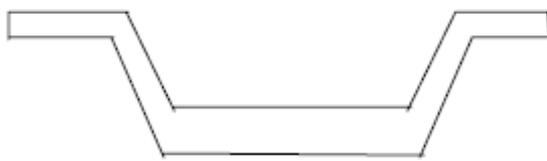
Mould is made from foam, with a layer of plaster to prevent matrix from seeping into the foam. The mould surface is smoothen and filled for a good finish.
