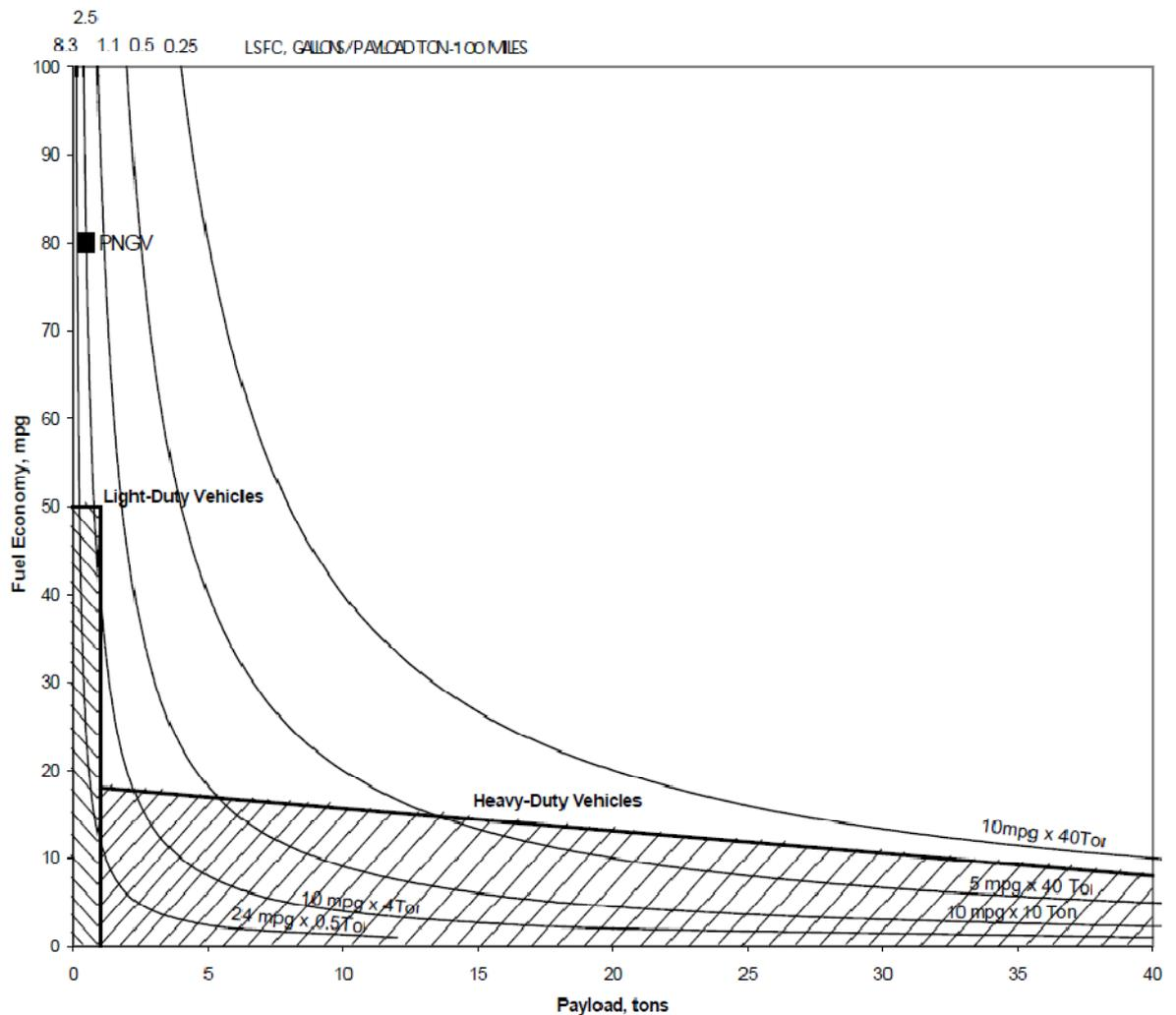
Figure 2: Relation between the fuel efficiency and weight of vehicle.
