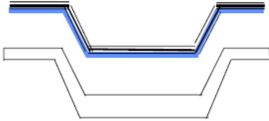
Once the composite is fully cured, it can be easily removed from the mould.
