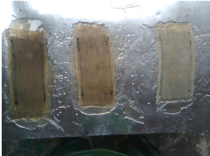
Figure 34: The fibreglass composites that are hardening.
