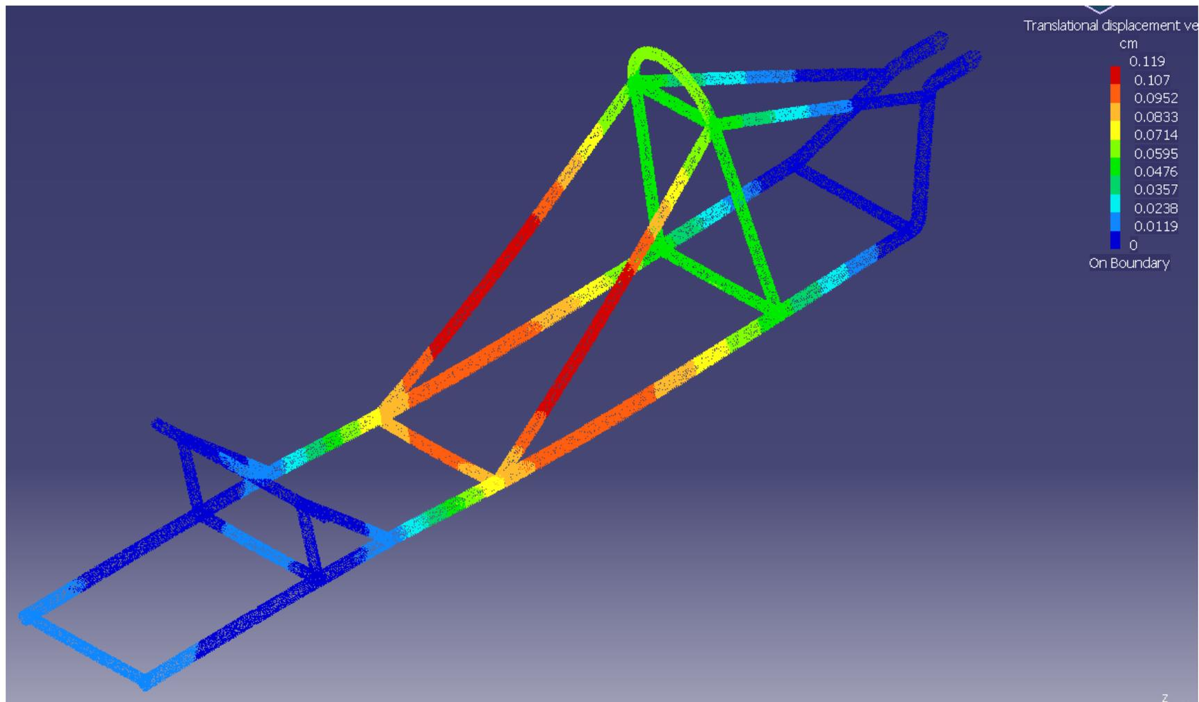
**Deflection of Frame with Braking Load**
