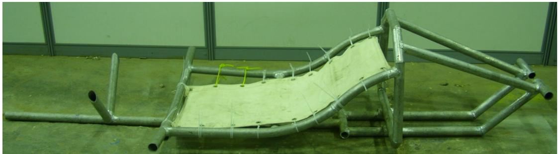
Figure 7: IUT's backbone frame.
