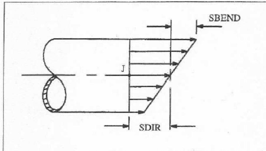
Figure 12: Bending stress
