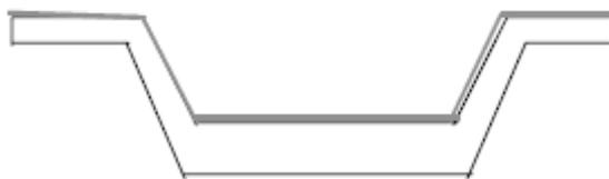
Mould release agent such as wax or silicon is applied onto the mould area.
