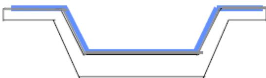
The woven fibreglass is cut according to the mould shape and placed onto the mould. The resin matrix is then poured onto the fibreglass. The composite is evenly applied using a roller.
