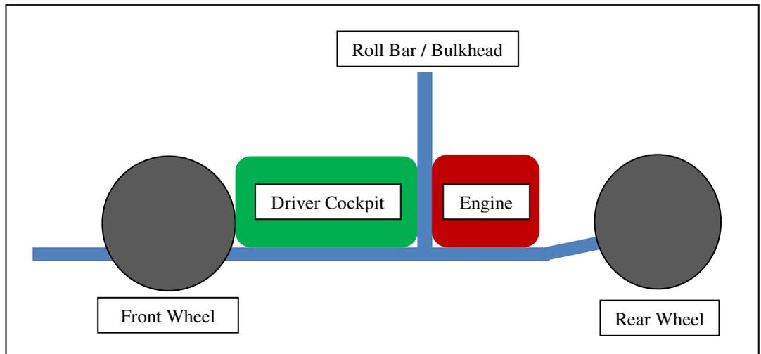
Figure 21: Basic layout of frame design
