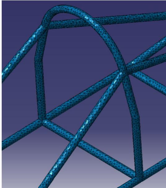
Figure 25: Close –up of meshing of nodes and elements
