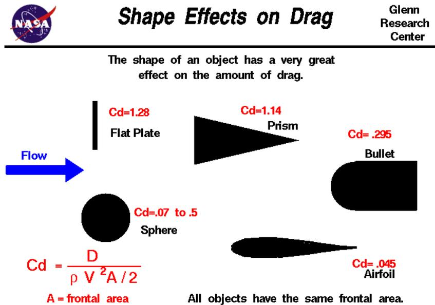
Figure 30: Drag Coefficient of various shapes
