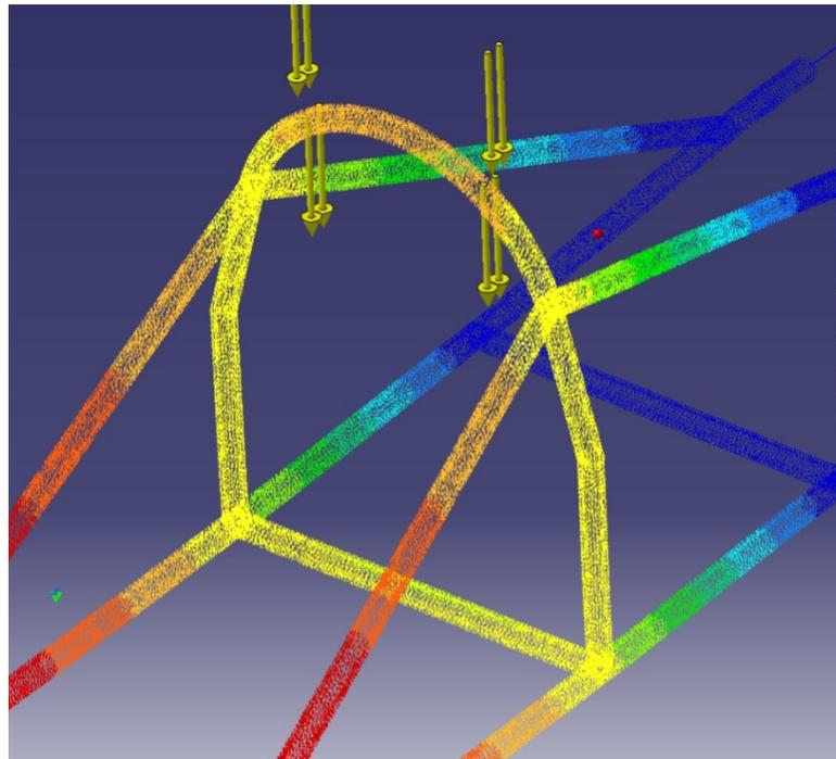
Figure 28: Deflection of roll bar under 700N load
