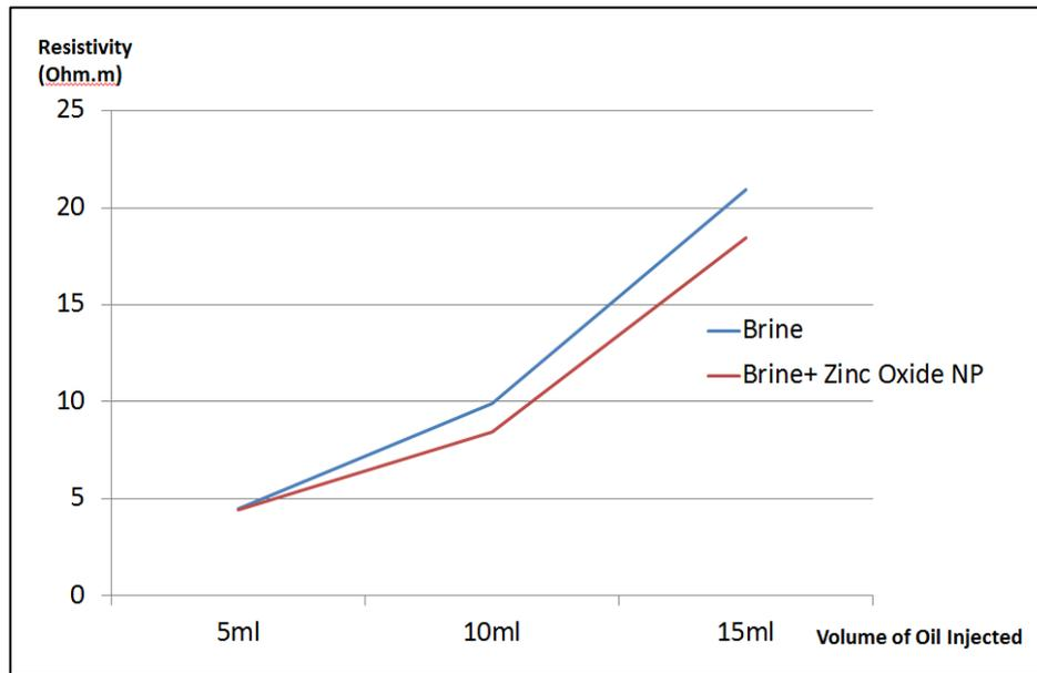
Figure 12: Resistivity of sand pack with different crude oil concentration
