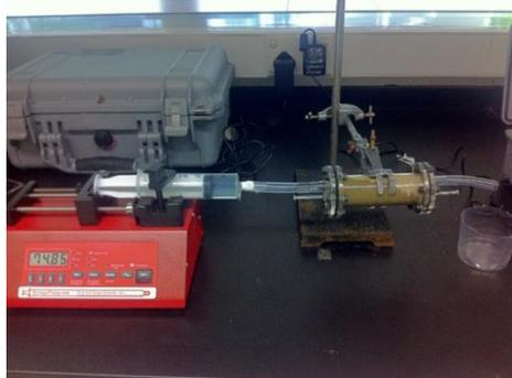
Figure 6: Sand pack experiment set up
