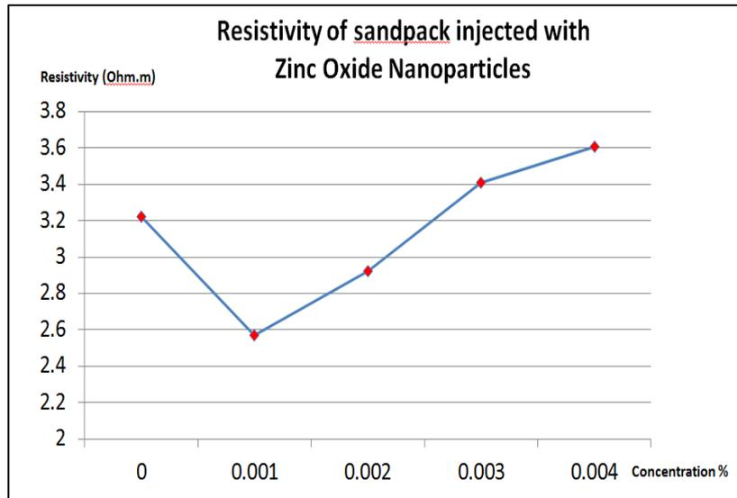
Figure 10: Resistivity of sand pack injected with different concentration of Zinc Oxide
