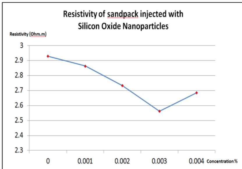
Figure 11: Resistivity of sand pack injected with different concentration of Silicon Oxide
