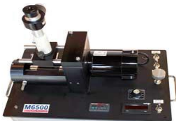
Figure 6 - Spinnig Drop Tensiometer
