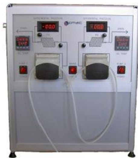
Figure 3 - PMAC Wax Appearance Temperature Apparatus
