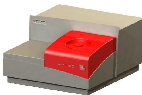
Figure 5 – micro Differential Scanning Calorimeter
