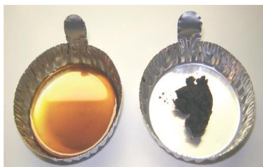
Figure 4 - Crude oil sample above WAT (left) and crude oil sample below WAT (right)
