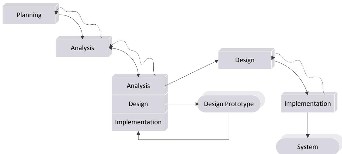
Figure 3.1. Throwaway prototyping-based methodology
