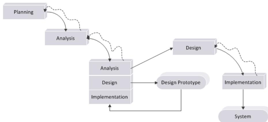
Figure 9. Throwaway prototyping based software development methodology
