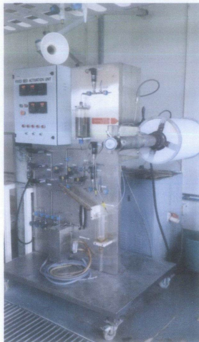
Figure 8: Fixed bed activation unit
