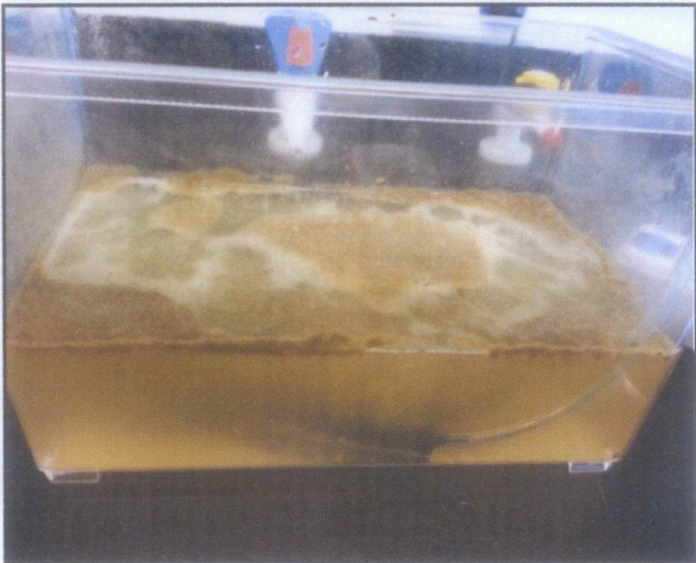
Figure 4.4: Dissolved Air Floatation on 10 th minutes (high intensity of bubbles)
