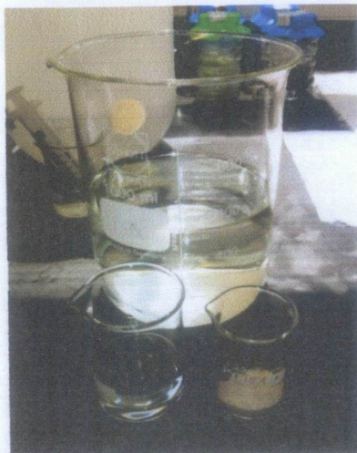
Fig. 3.3: Synthetic MEA wastewater in 1 L beaker, and hydrogen peroxide and iron(II) sulphate in 50 ml and 25 ml beaker
