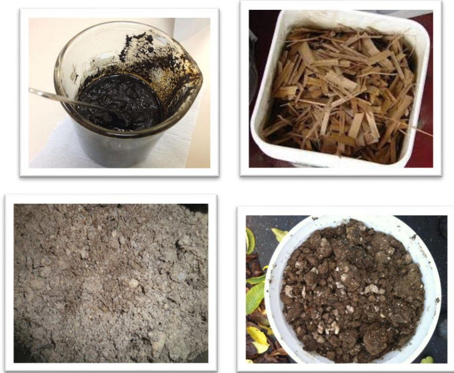
Figure 3: Materials used for this study (Oil Sludge, Soil, Palm Frond, and Manure)
