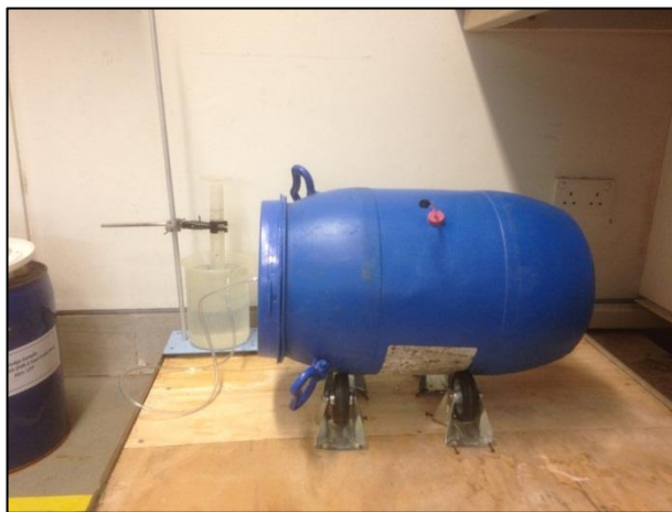
Figure 2: Designed Prototype of Compost Tumbler
