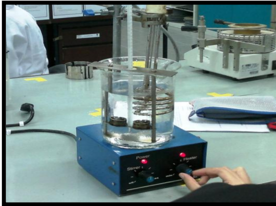
Figure 3.5: the water bath temperature must be control at uniform rate ( 5.0 \pm 0.5^{\circ} per minute)
