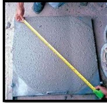
Figure 16: Slump Flow measurement
