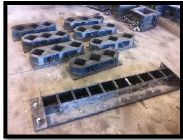
Figure 12: The moulds prepared for the mix
