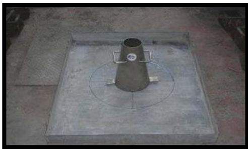
Figure 14: T-50 slump flow
