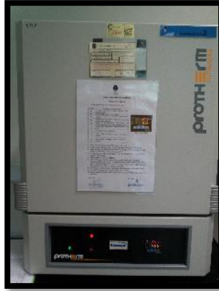
Figure 17: Protherm Furnace for heating of samples
