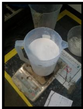
Figure 8: 99.5% Pure Nano Silica Powder
