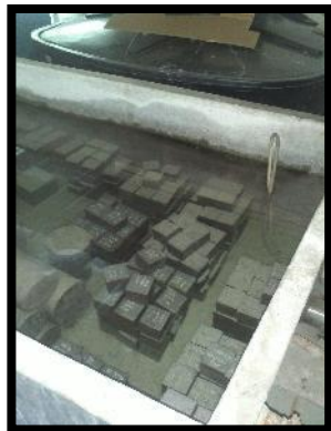
Figure 13: The concrete cubes in curing tank
