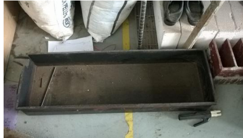
Figure 6. Hydrocarbon pool tank
