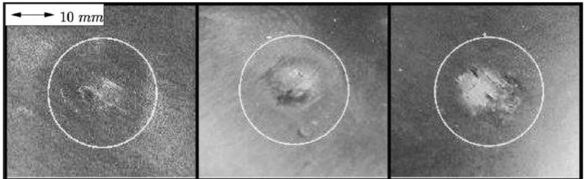
**Figure 16:** Effect of the temperature on the impacted side damage. Quasi-isotropic laminate impacted at 5 J. 20 (left), 260 (center) and 2150 8C (right)[14].
