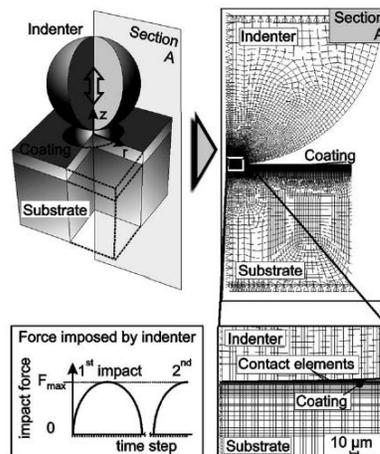
**Figure 37:** The developed impact test FEM model with deformable ball indenter.
