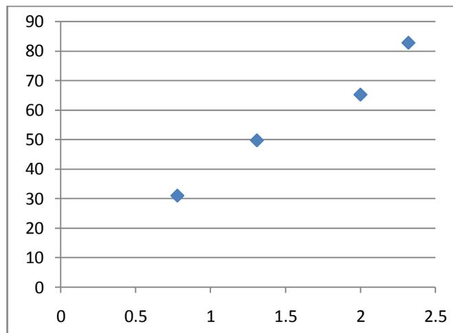
**Figure 36:** Impact Force vs. Impact Depth graph
