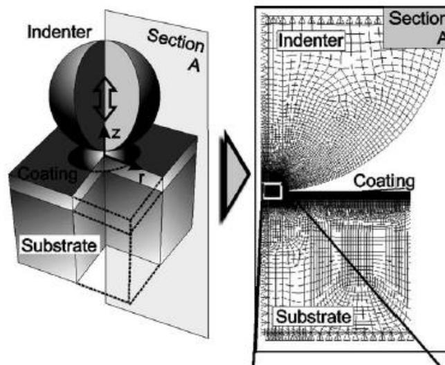
**Figure 6:** The cross section of the indenter and the impact zone at the coating [9].
