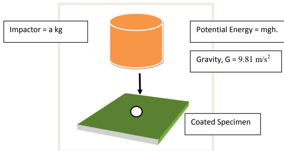
**Figure 10:** The impact test free body diagram
