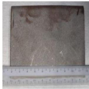
**Figure 17:** Cold rolled substrate after been prepared with SA2.5 industrial standards. After the surface preparation has been done, the coating application process took place.
