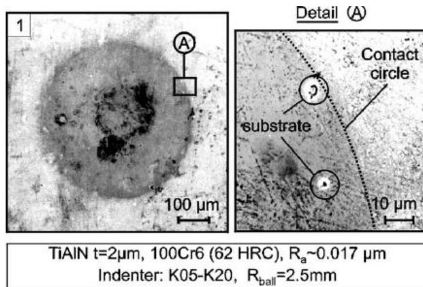
**Figure 11** : Failure initiation of a TiAlN coating on a smooth surface deposited
