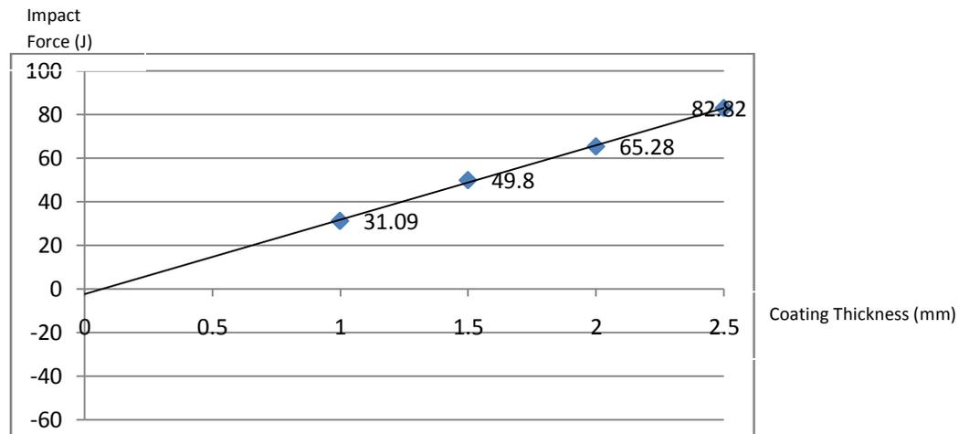
**Figure 35:** Impact Force vs. Coating thickness graph.
