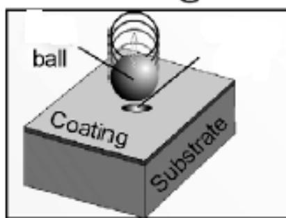
**Figure 5:** The examples on how the weight will drop onto the lying punch on the surface of the coating, thus indent the coating. Notice the test was done by the intrusion method (coating facing upward)
