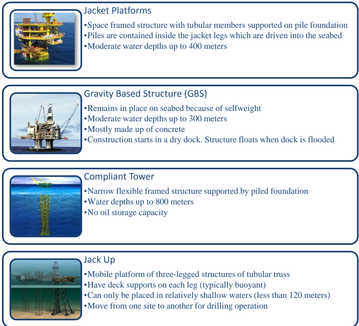
Figure 2: Fixed structures of offshore platforms
