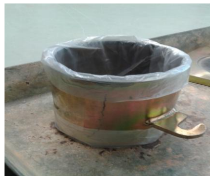
Mould covered with plastic
