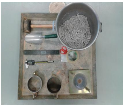
Apparatus for compaction
