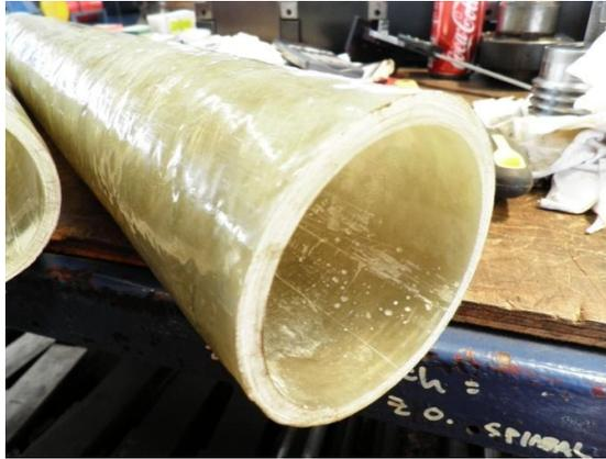
**Figure 4.8: Effects of air bubbles inside the pipe**
