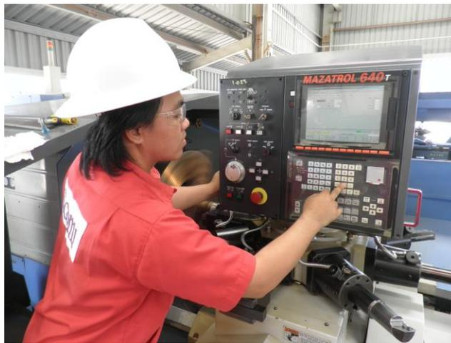
**Figure 3.6: Technician is conducting pre-adjusting on the machine**
