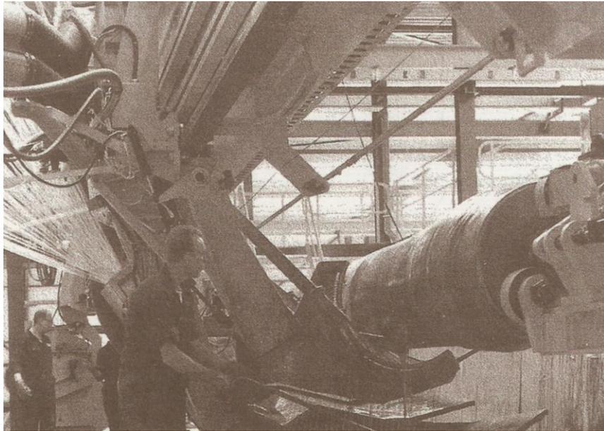
**Figure 2.6: Filament winding machine with large diameter mandrel (courtesy of Owen (2000))**
