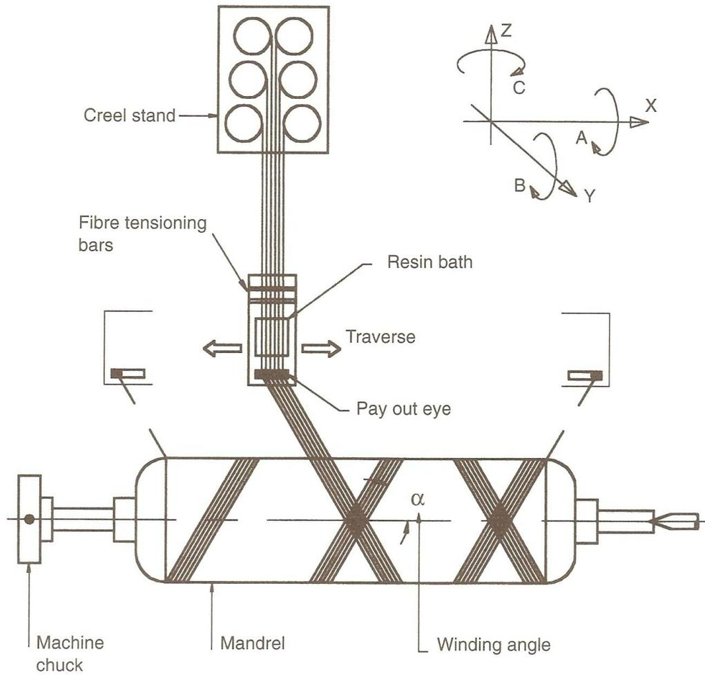
**Figure 2.4: Schematic Presentation of Filament Winding Process**
