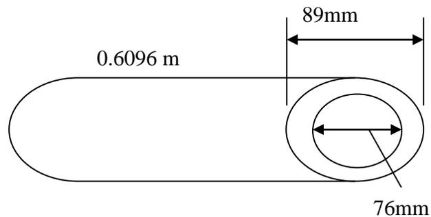
**Figure 4.1: Proposed dimensions for composite pup joint**
