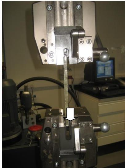
**Figure 4.13: Friction grips hold and tightened test specimen in place**
