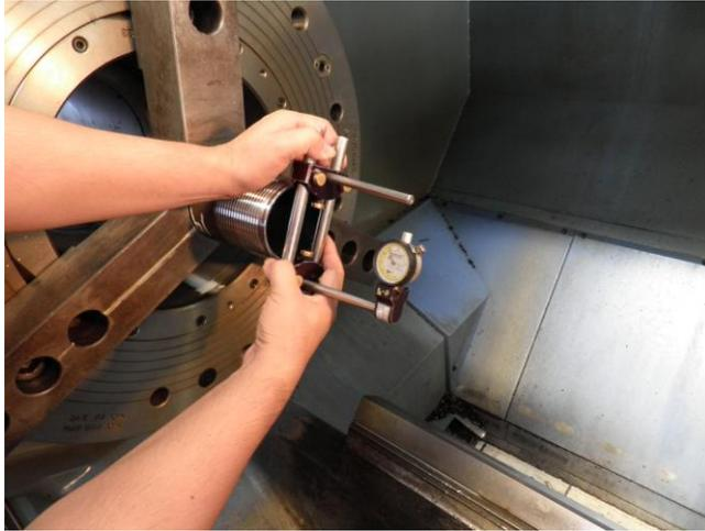
**Figure 3.7: Measure the OD of the thread sealing area using a gauge**
