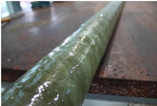
**Figure 4.6: Rough surface finish of pipe's outer surface**
