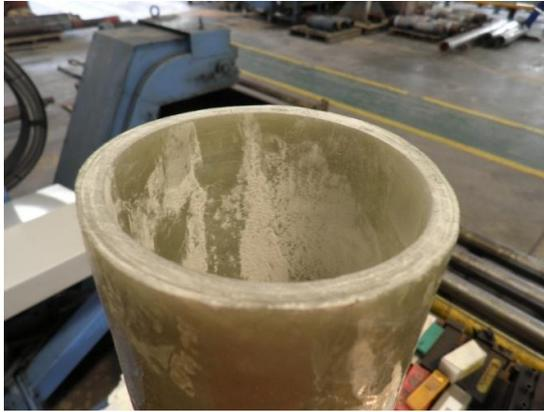
**Figure 4.7: Releasing agent powder in pipe**
