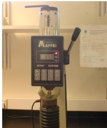
**Figure 4.11: Hardness is measured to the pipe wall thickness**
