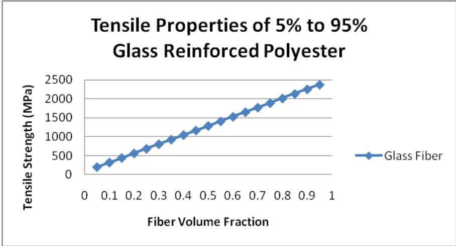
**Figure 4.3: Graph of tensile strength versus fiber volume fraction**
