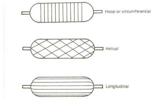
**Figure 2.5: Three types of pattern available from filament winding process**
