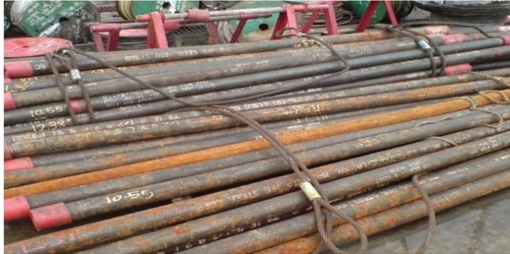
**Figure 1.1: Corroded low alloy steel pup joint**
