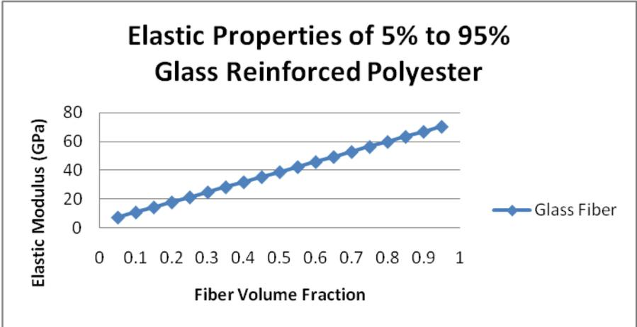
**Figure 4.2: Graph of elastic modulus versus fiber volume fraction**
