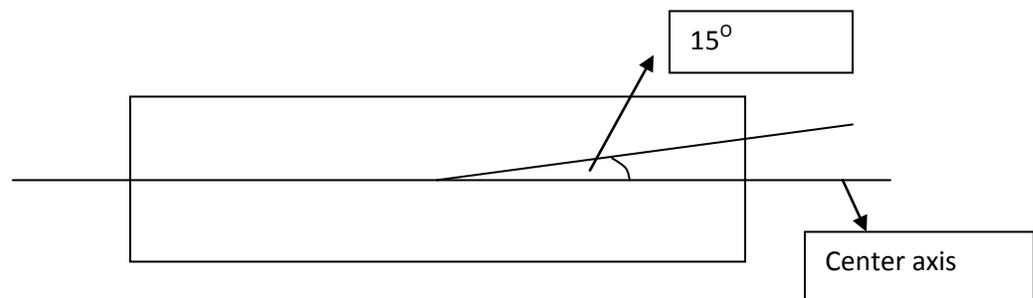
**Figure 4.4: Winding pattern of pup joint**
