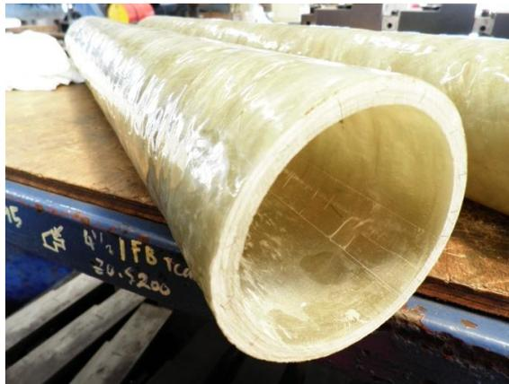
**Figure 4.9: Line scratches are closed to each other inside the pipe**
