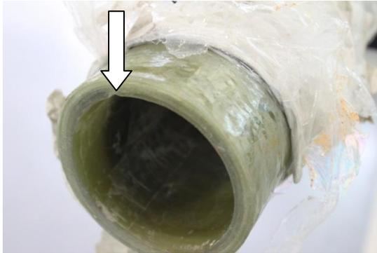
**Figure 4.5: The arrow shows the crack area**
