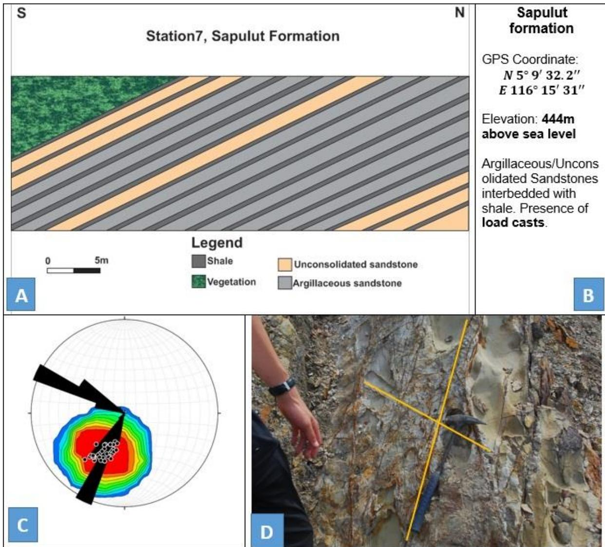
**Figure 37 : ILLUSTRATION OF THE OUTCROP, LITHOLOGY DESCRIPTION, STERONEET AND CONJUGATE JOINTS OF STATION 7, SAPULUT FORMATION.**
