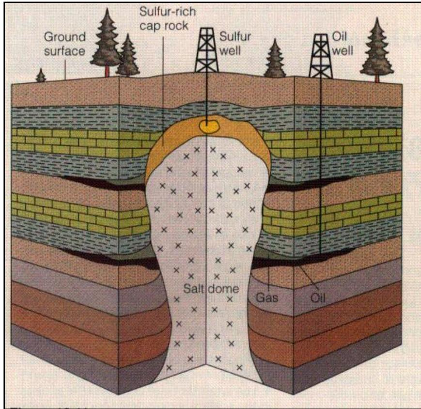
Figure 4 :SCHEMATIC 3D DIARGAM OF THE SALT DIAPIR/DOME.
